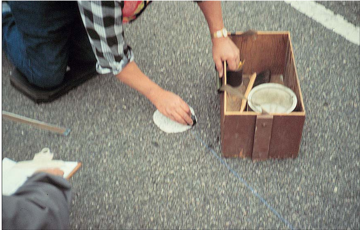
Figure 3-2. MEASUREMENT OF MACRO TEXTURE DEPTH USING ASTM E 965 – 96.
