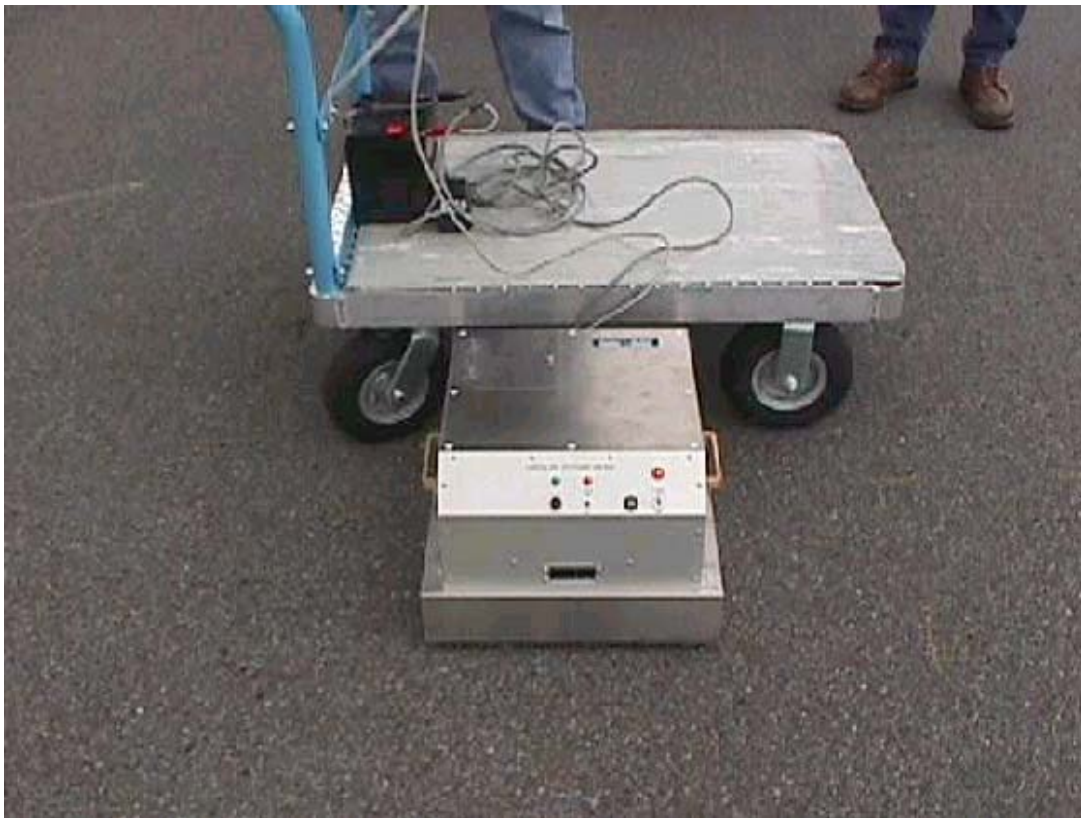
Figure 3-3. APPARATUS FOR MEASURING SURFACE MACRO-TEXTURE DEPTH
