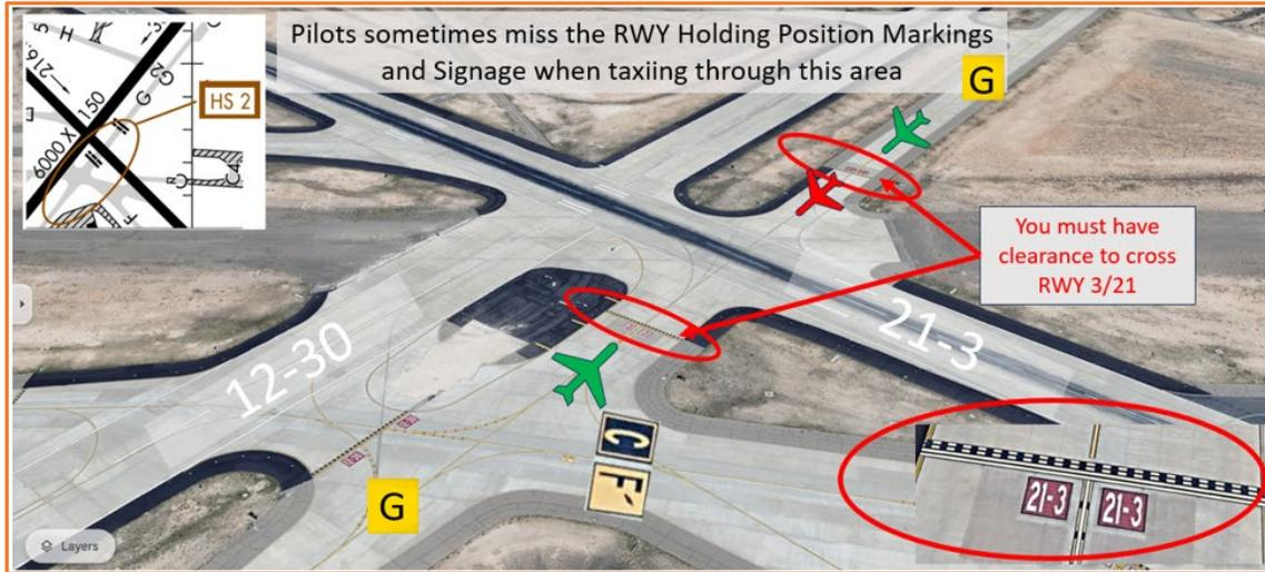
**HS 3** TWY E5 permanently closed. Hold short lines for RWY 3/21 on TWYs E, H, and Hot Pad 2. Risk to pilots traveling on TWY E of confusing TWY H and RWY 3/21.
