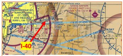
The "East Pass" Departure Route from Albuquerque (KABQ) typically follows the I-40 corridor and is designed to help pilots navigate the mountainous terrain to the east of the city.
