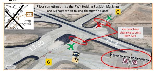
HS 3 TWY E5 permanently closed. Hold short lines for RWY 3/21 on TWYs E, H, and Hot Pad 2. Risk to pilots traveling on TWY E of confusing TWY H and RWY 3/21.
