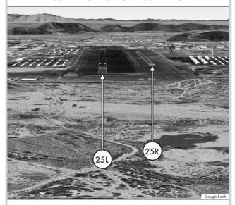
Offset parallels; RWY 25R is 650 feet farther down the approach than RWY 25L. Pilots sometimes confuse RWY 25L for RWY 25R.
