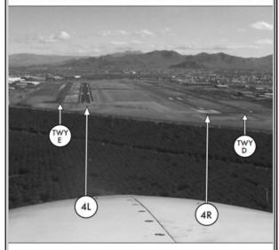
Offset parallels; RWY 4L is 500 feet farther down the approach than RWY 4R. Pilots sometimes confuse RWY 4R for Runway 4L, TWY D for RWY 4R or TWY E for RWY 4L.
