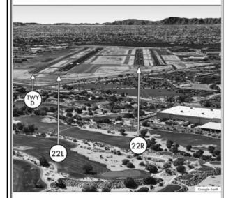
Offset parallels; RWY 22R is 750 feet farther down the approach than RWY 22L. Pilots sometimes confuse RWY 22L and Runway 22R, or TWY D for RWY 22L.
