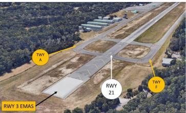
RWY markings are white. Markings on surfaces not used for takeoff/landing like TWY markings, chevrons, RWY shoulder and RWY turn-on markings etc., are yellow.
