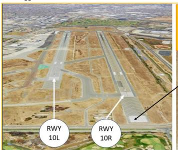
RWY 28L Engineered Materials Arresting System (EMAS) which uses crushable material placed at the end of a runway to help stop an aircraft that overruns the runway end.
