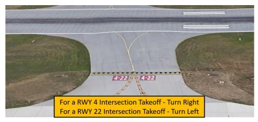
✓ Prior to entering the RWY and again when lining up on the RWY, check your Magnetic Compass and, (if installed), your Horizontal Situation Indicator (HSI) to verify that you are pointed in the correct direction.
