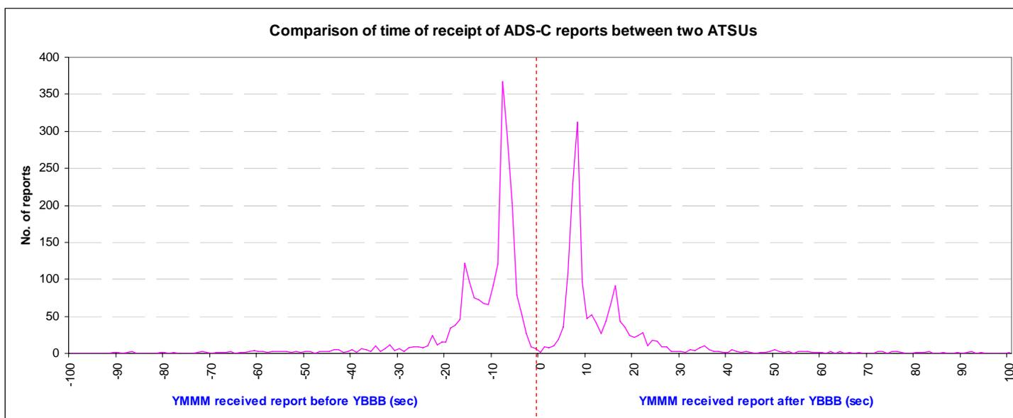
**Figure1. Graph comparing transmission delays for identical ADS-C reports**
