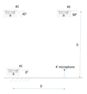
Figure 1. Sketch of supplemental hover test conditions. D = 20 feet.
