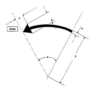
Arrow point and base of arrow shaft to be within 25 mm (1 inch) of fully unlocked and fully locked positions respectively
