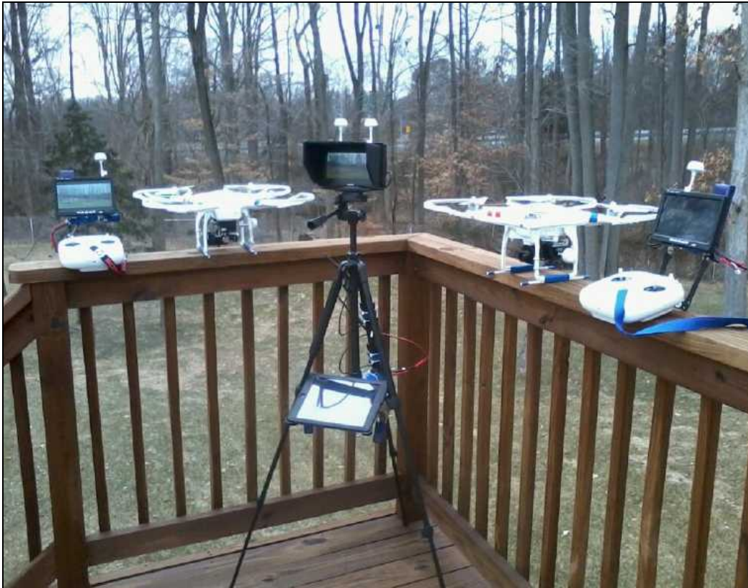
Figure 1. DJI Phantom 2 quad-copters with Radio Controllers and either a GoPro Hero3+Black camera or a FLIR Tau 2 camera. A tripod-mounted Ground Control Station with separate higher-resolution viewing screen is also shown.
