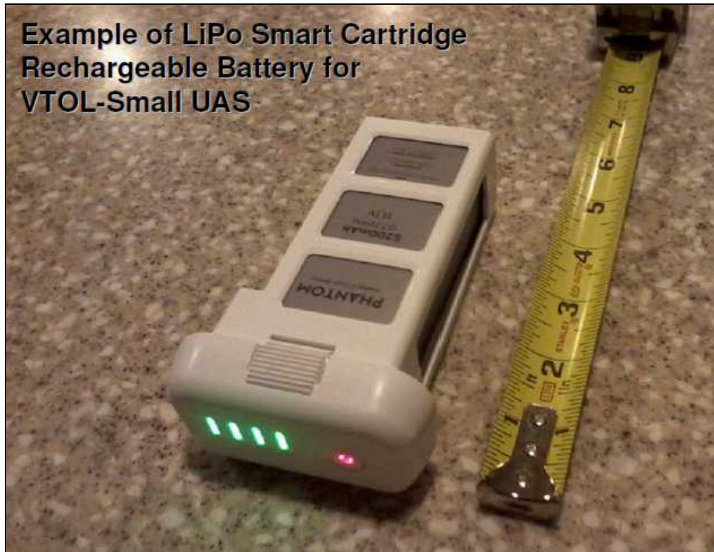
Figure 4. Smart Battery employed in Phantom 2 provides immediate visual awareness and percent battery charge remaining as well as similar information during flight through Ground Control Station.
