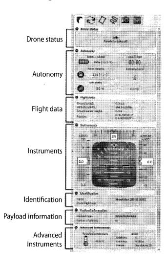
The Flight Monitoring tab can be used to monitor the *eBee* during a mapping mission and is the default tab that is displayed when you click anywhere on the map area that does not have a symbol. The tab is split into the following sections:
