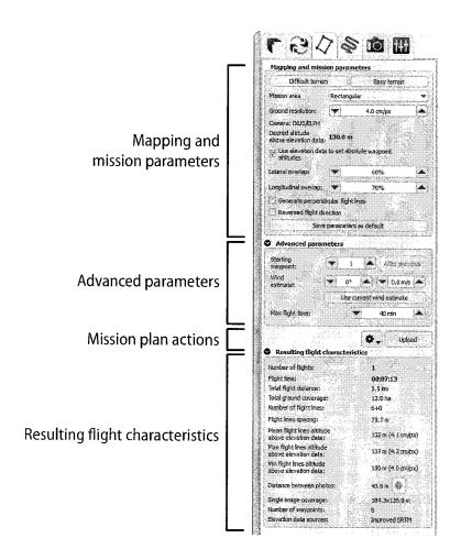
The Mission Planning tab is divided in several panels. The first panel, **Mapping** and mission parameters, contains the parameters that define the requirements of a particular mission:
