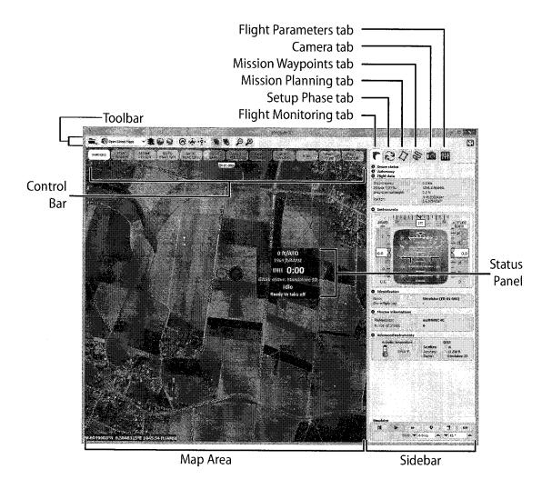
The main *eMotion* interface is composed of a Map Area, a Toolbar and a Sidebar<sup>29</sup>. The Map Area displays the current location of the *eBee*, a Status Panel with important information on the drone's current status, and a Control Bar used to send commands to the drone (section 'Control Bar' on page 89).
