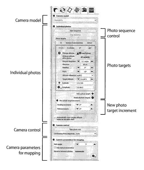
The camera tab is an advanced tab that can be used to precisely control the functioning of the camera. It also contains controls for taking oblique imagery. It is split into several sections: 'Camera model', 'Photo targets', 'Camera control', and 'Camera parameters for mapping'.
