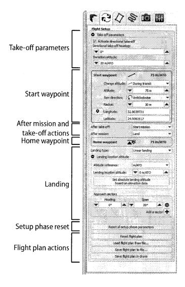
The Setup Phase tab is used to define the setup phase of a flight plan. This phase includes the definition of the Home and Start waypoints and the actions to be taken before and after the mission phase of the flight plan.
