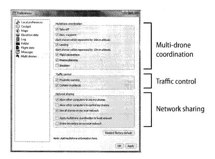
*eMotion* provides Multi-drone coordination options to synchronise various way-points and parameters among connected drones:
