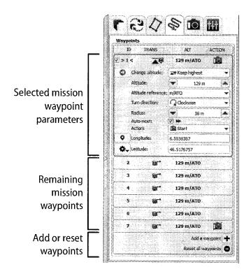
The Mission Waypoints tab contains a list of all mission waypoints currently on the drone autopilot. It can be used for finer control of individual waypoints in the current mission. The list of waypoints displays the ID, Change altitude parameter, Altitude and Action related to each mission waypoint.
