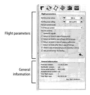
The Flight Parameters tab includes some advanced functions that govern the overall behaviour of the drone while in flight. It is separated into two sections: 'Flight parameters' and 'General information'. The 'Flight parameters' section includes the following items:
