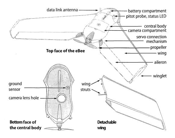
The eBee is an autonomous flying drone comprised of the following components:
