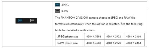
RAW is not supported in continuous capture mode or timed capture mode. JPEG photos will be created automatically.
