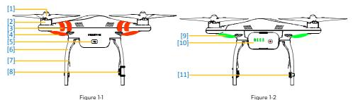
[1]Propeller [2]Motor [3]Front Side [4]Front LEDs [5]Micro-USB Port [6]Landing Gear [7]Receiver
