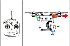
The left dial controls the pitch of the H3-2D and H3-3D gimbal. The position of left dial determines the pitch angle relative to the horizontal level.
