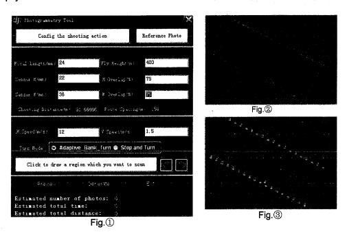
STEP1: Click ToolBox > Photogrammetry Tool to open the setting window, shown as Fig. 1.
