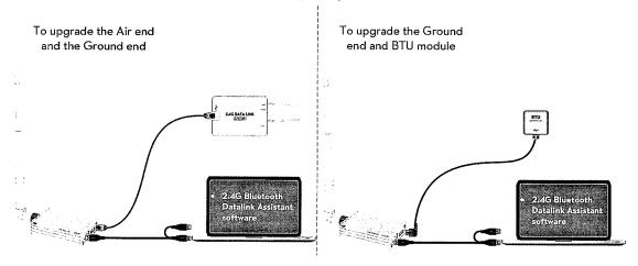
Important: POWER CYCLE the Flight control system and 2.4G Bluetooth Datalink after upgrade.
