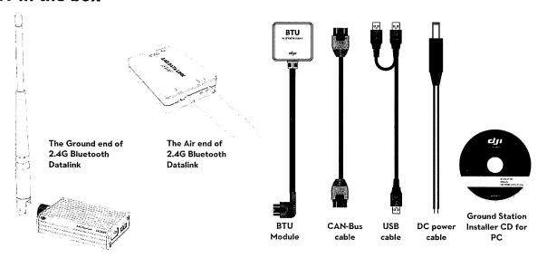
Important: the firmware of BTU should be upgraded to version 1.0.1.2 or above to use with the 2.4G Bluetooth Datalink.
