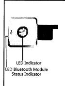
The LED Bluetooth Module is necessary if you are using the WM Assistant. This module is only for the iOS Device, not for android equipment. Its Operating Temperature range is from -5°C to +60°C. Please refer to the Assembly & Configuration -> Step1 Assembly to attach the module.
