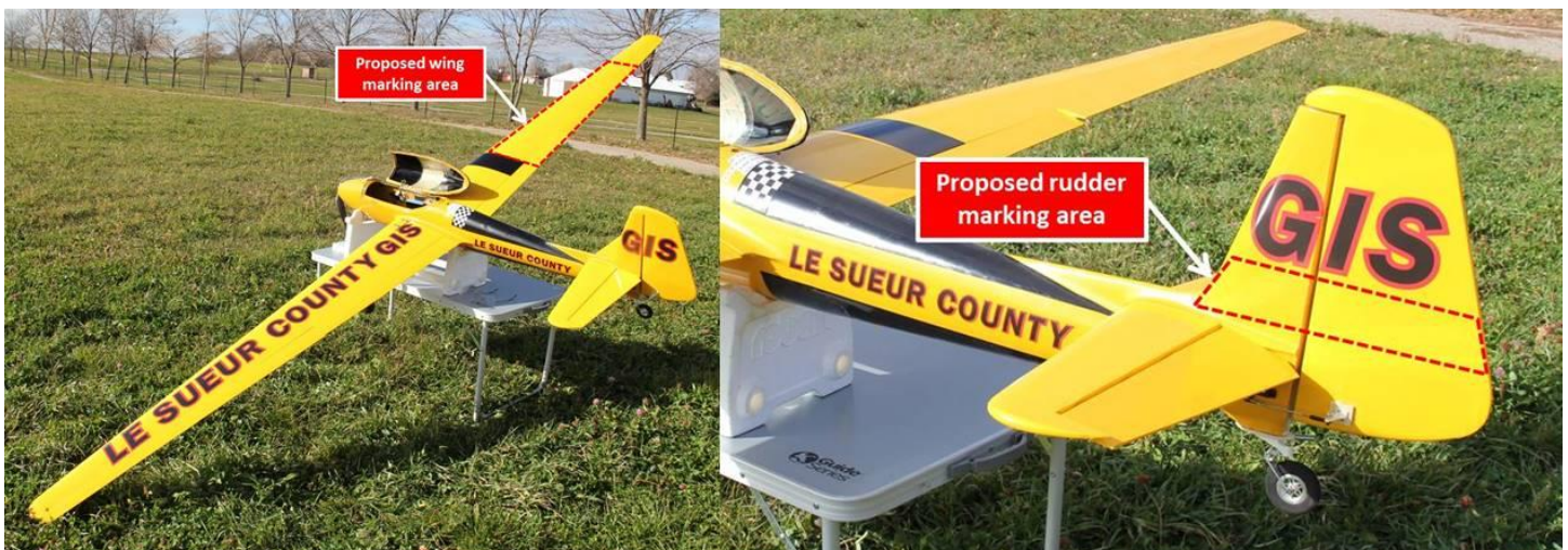
Proposed “N” Number Marking Locations – (Pending Approval with FAA)
