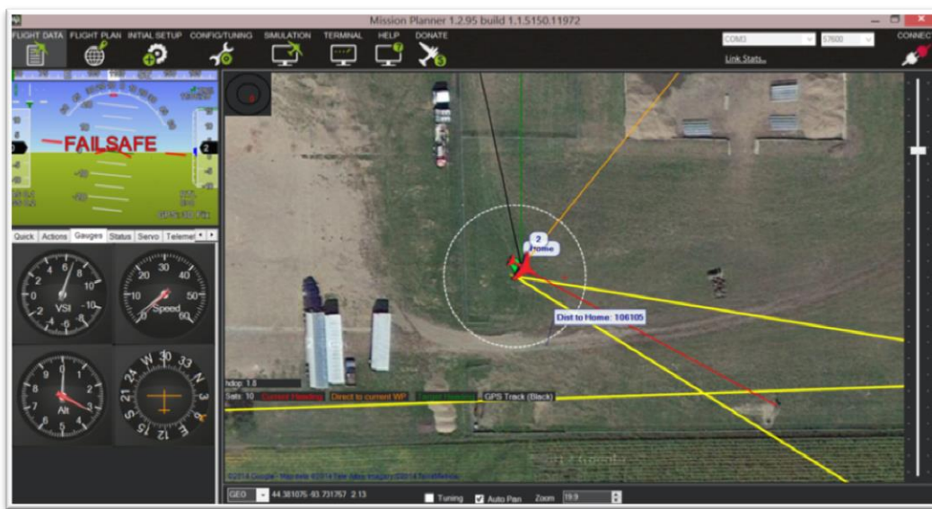
Telemetry Computer Display - Primary RC Link Fail-Safe Indication
