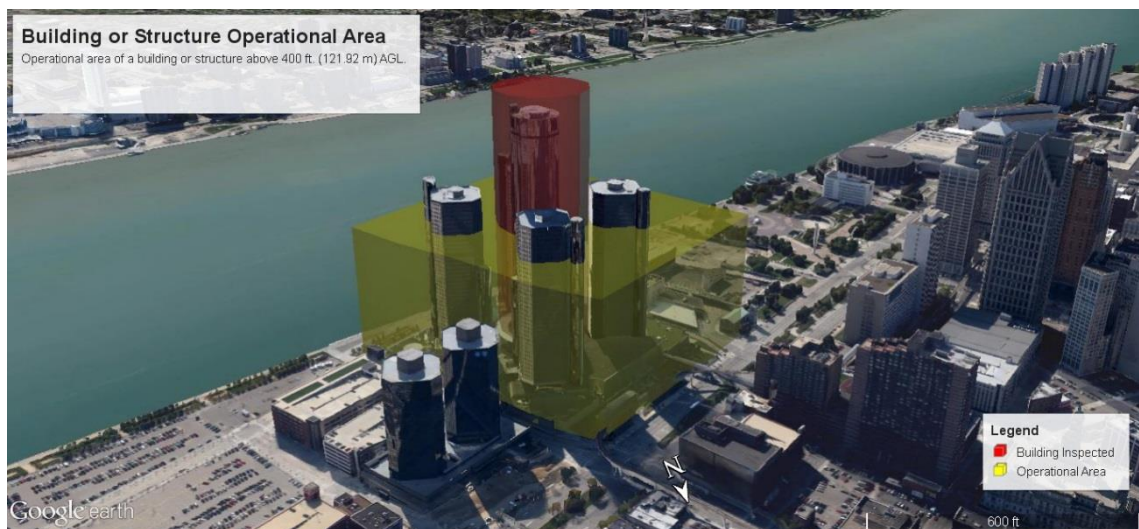
Fig. 4.1 Operational area around a building taller than 400 ft. (121.92 m) AGL. Note the area around the perimeter of the property only extends to 400 ft. (121.92 m) AGL. Also note the North side of the operational area does not extend over the highway.
