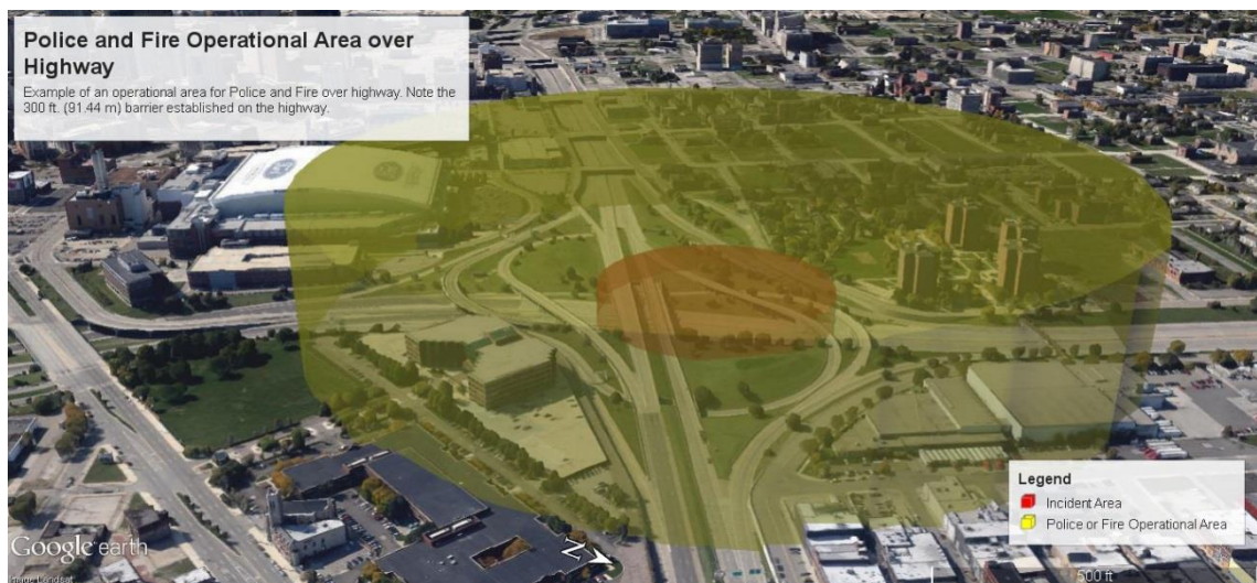
Fig. 7.3 Operational area over highway. Due to the nature of hazardous or explosive cargo sometimes shipped over highways, an sUAS may have to enter anywhere from up to 1000 ft. (304.8 m) away for increased safety to the Equipment Operator and Spotter. Note the 300 ft. (91.44) barrier established in the Incident Area depicted in red.
