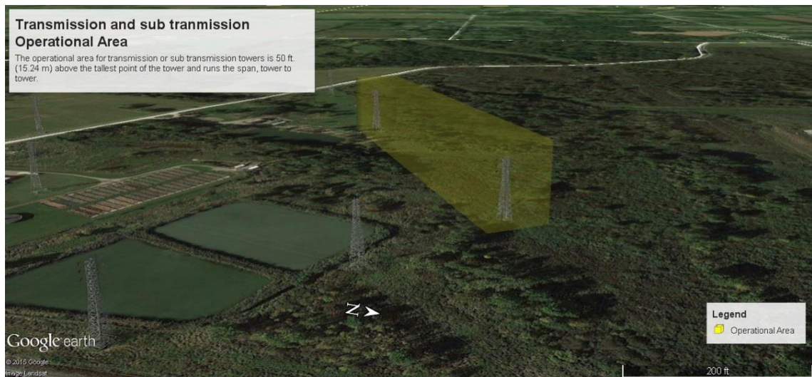
Fig. 3.2 Operational area for transmission and sub transmission Towers.
