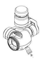
O Do not remove micro-SD card from the Inspire 1 when it is powered on.
