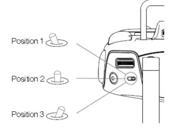
P-mode (Positioning): P-mode works best when the GPS signal is strong. There are three different versions of P-mode, which will be automatically selected by the Phantom 3 Professional depending on GPS signal strength and the Vision Positioning sensors:
