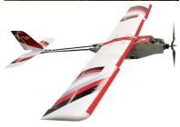
The Hawk is a battery-powered drone allowing flight times up to 40 minutes. Its wingspan is 48 inches. Takeoff weight is 3 pounds.
