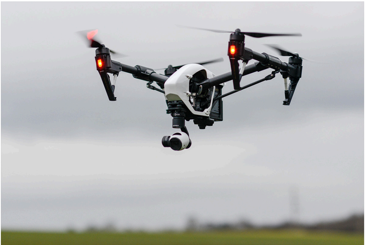
FIGURE 1: INTERNATIONAL-WIND'S INSPIRE 1 WITH BUILT IN VIDEO/CAMERA SYSTEM
