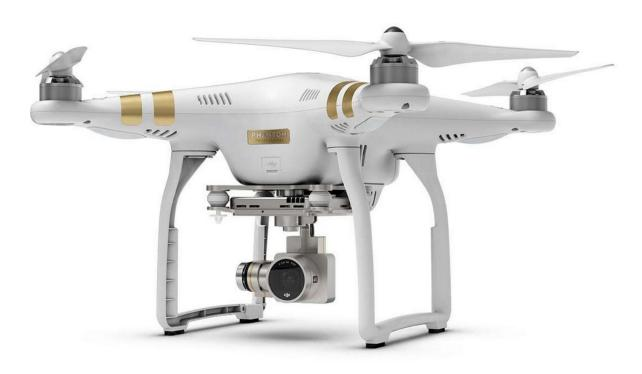
Aircraft Weight (Including Battery And Propellers): 1280g
