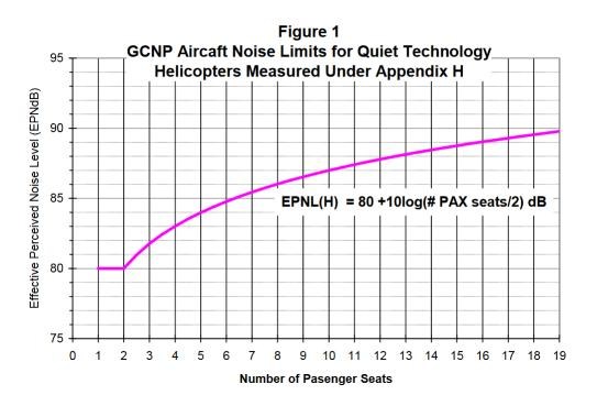
The vertical axis is the noise level; the horizontal axis is number of passengers. Aircraft that fall below the pink line qualify as quiet technology. The pink line defining quiet technology is actually a function of the number of passenger seats on the aircraft. In the equation, the independent variable is passenger
