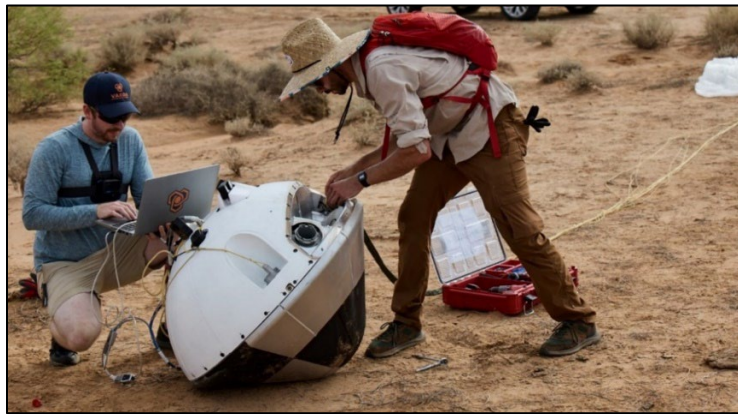
Figure 2.1-6. Recovery of the Varda Capsule and Main Parachute after a 2022 Parachute Test in Arizona
