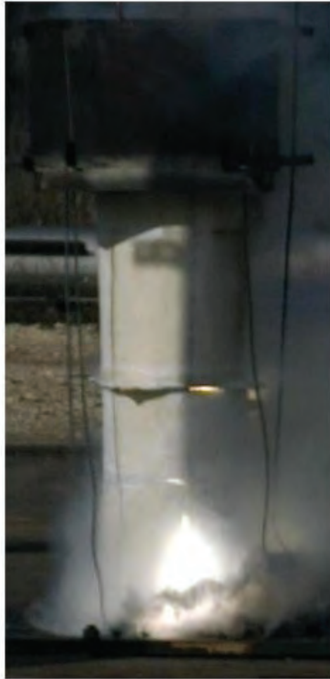
Figure 2: SN9 Transfer Tube Failure of TXC-4907-08
