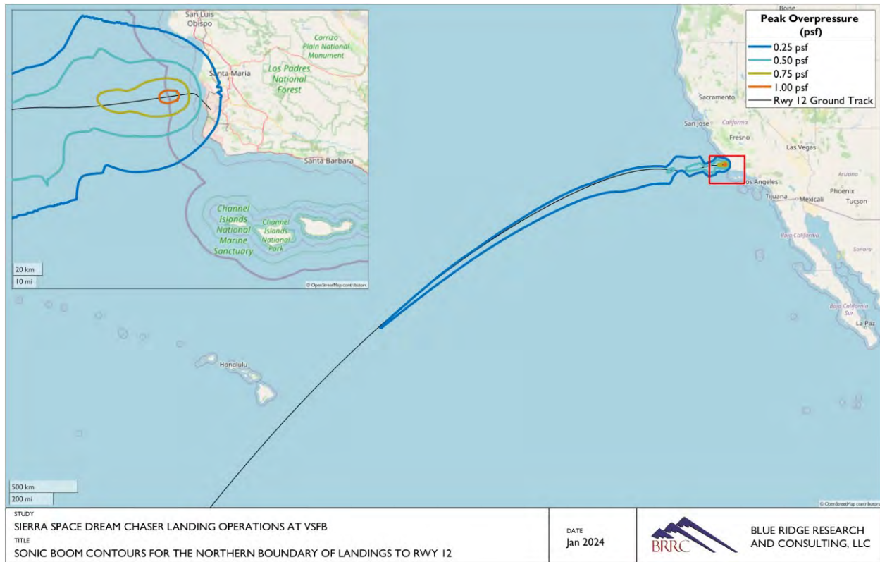
Figure 4. Sonic boom contours for the northern boundary of landings to Runway 12.
