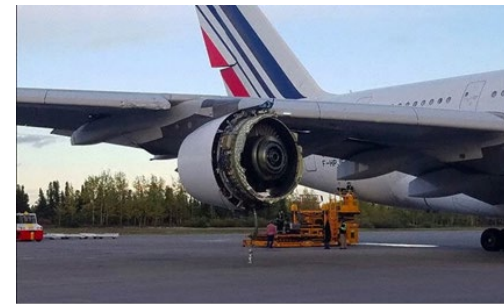
AF Flight 66 Titanium “Cold Dwell Fatigue”
