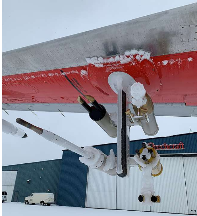
Instruments attached to the wing--including (counterclockwise from upper left) a forward scattering spectrometer probe, Rosemount air data probe, and cloud droplet probes--measure different cloud particle sizes and concentrations.
