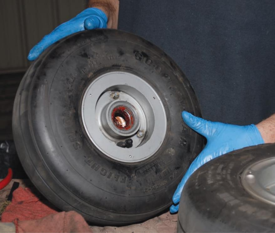
**Preventive maintenance tasks include the removal, installation, and repair of landing-gear tires, as well as cleaning and greasing wheel bearings.**
