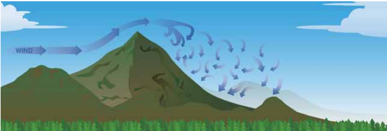
Paying attention to wind direction and avoiding flying near the leeward side of mountains can help avoid the turbulence illustrated here.
