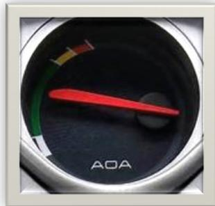
An AOA indicator can be used to get the pilot’s attention (via audio and/or low cost stick shakers) even if the pilot is not looking at it. This focuses the pilot’s attention on where it needs to be to avoid the stall. It can also help when used in conjunction with airspeed and existing stall warning systems, when available.
