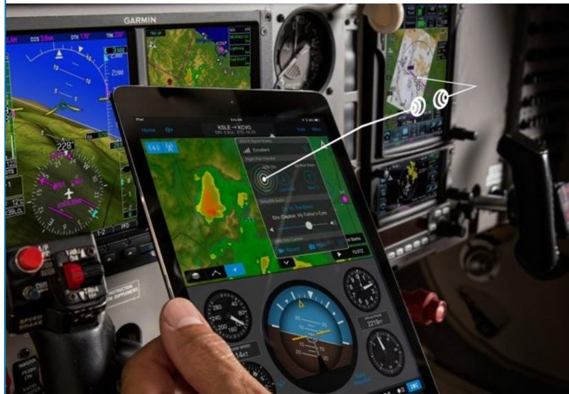
Interconnected devices and sensors make more information available in the cockpit than ever before. Air/Ground data links can provide ATC clearances and instructions as well as weather depiction and field condition reports and NOTAMS.
