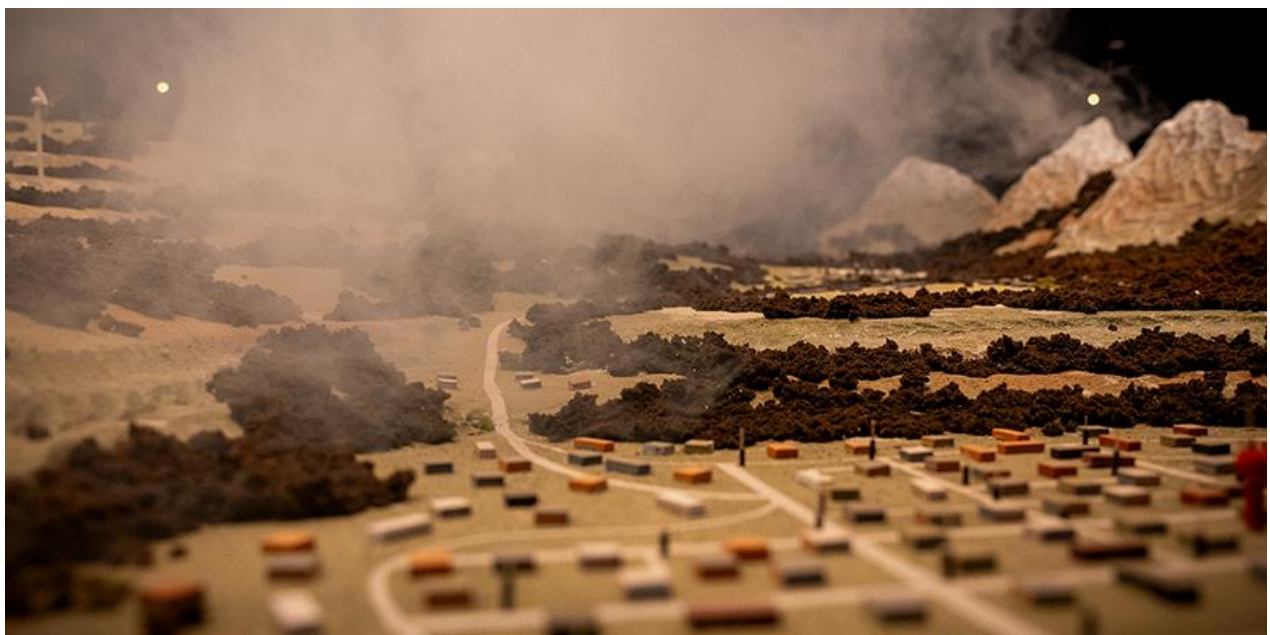
Theatrical smoke is added to the demo. The smoke helps to demonstrate how particulates (rain, fog, smoke and dust) can adversely affect NVG functionality. The foreground shows a 1 – 600 scale city with foliage and white-capped mountains in the background.
