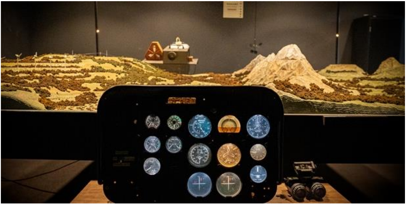
CAMI's NITE-Lab incorporates a functional helicopter instrument panel for a more realistic demonstration. In the background is scaled terrain board, smoke generator, and functional aircraft position lights.
