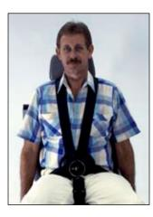
Shoulder harness systems can use dual shoulder belts or a single diagonal belt similar to those used in automobiles. The belts should not rub against your head or neck. This is uncomfortable, will discourage use of the shoulder harness, and can also cause neck injuries during an impact.
