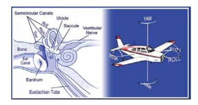
Each canal is filled with a fluid called endolymph and contains a motion sensor with little hairs whose ends are embedded in a gelatinous structure called the cupula. The cupula and the hairs move as the fluid moves inside the canal in response to an angular acceleration.
