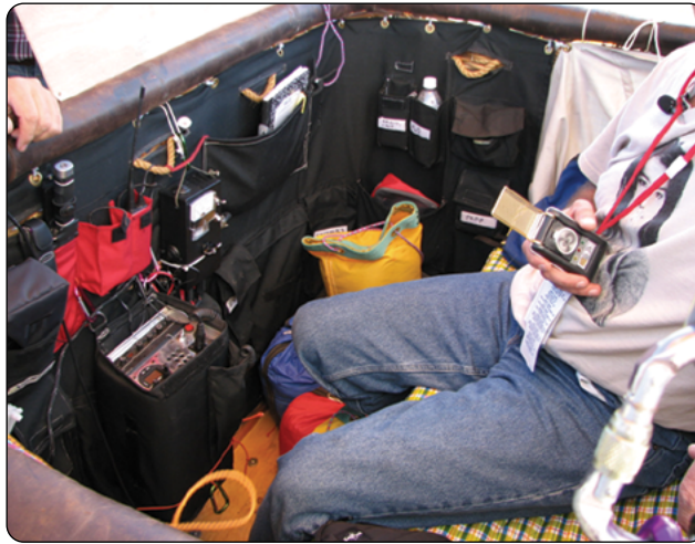
Figure 11-5. Typical gondola layout.
