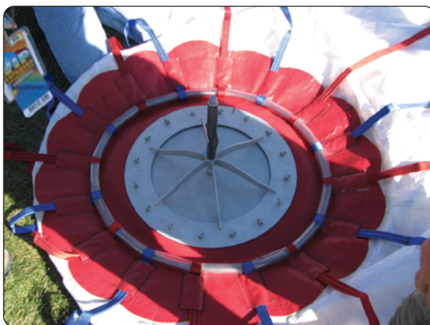
Figure 11-4. Maneuvering valve on quick fill gas balloon.
