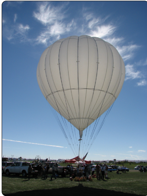
Figure 11-3. Quick fill design gas balloon.
