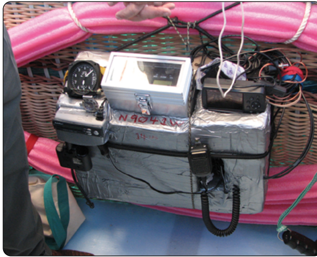
Figure 11-6. Instruments and radios are sometimes carried in a pod such as this.
