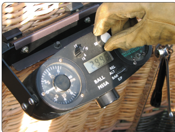
Figure 6-10. The altimeter should be set to barometric pressure, if available, or to the field elevation
