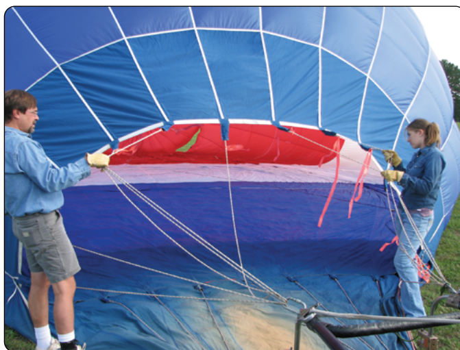
Figure 6-14. Determining correct inflation fan placement. Note that the strips of tape are generally pointing into the mouth. In this case, the pilot would do well to incline the fan slightly towards the right side of the mouth, in order to better “seal” the envelope opening, and get a more efficient inflation.
