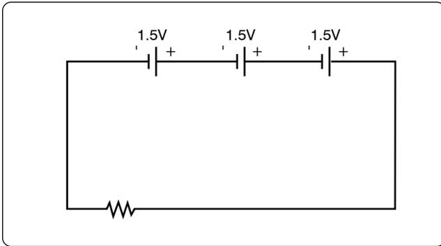
Figure 12-84. Voltage sources in series add algebraically.
