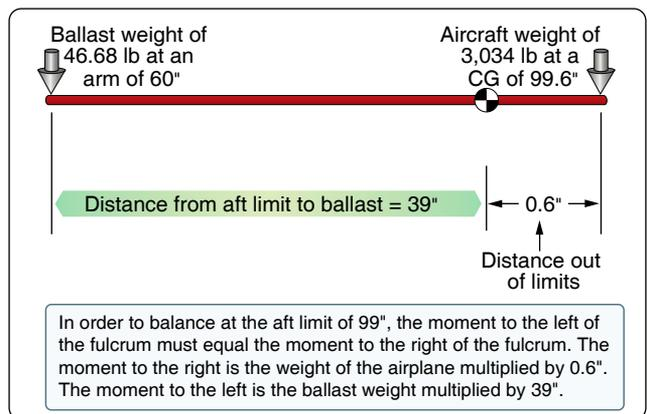
Figure 6-42. Ballast calculation as a first class lever.
