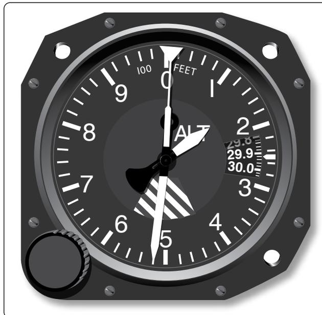
Figure 5-51. An airplane's altimeter is an aneroid barometer.
