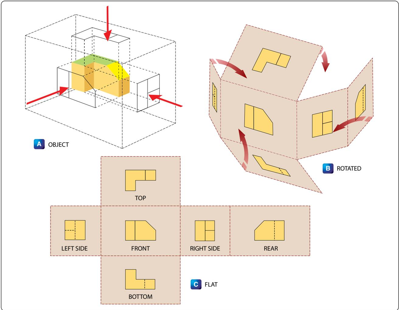
Figure 4-11. Orthographic projection.
