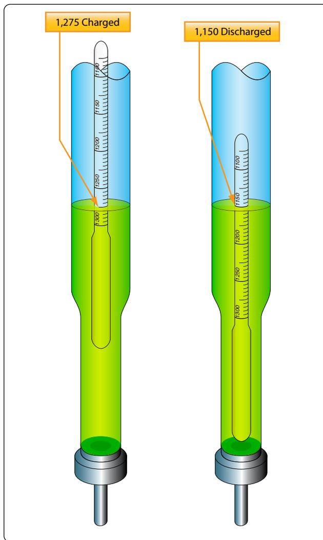
Figure 5-2. Hydrometer for checking battery specific gravity.
