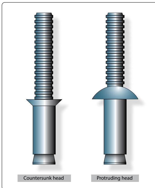
Figure 7-41. Pull-thru rivets.
