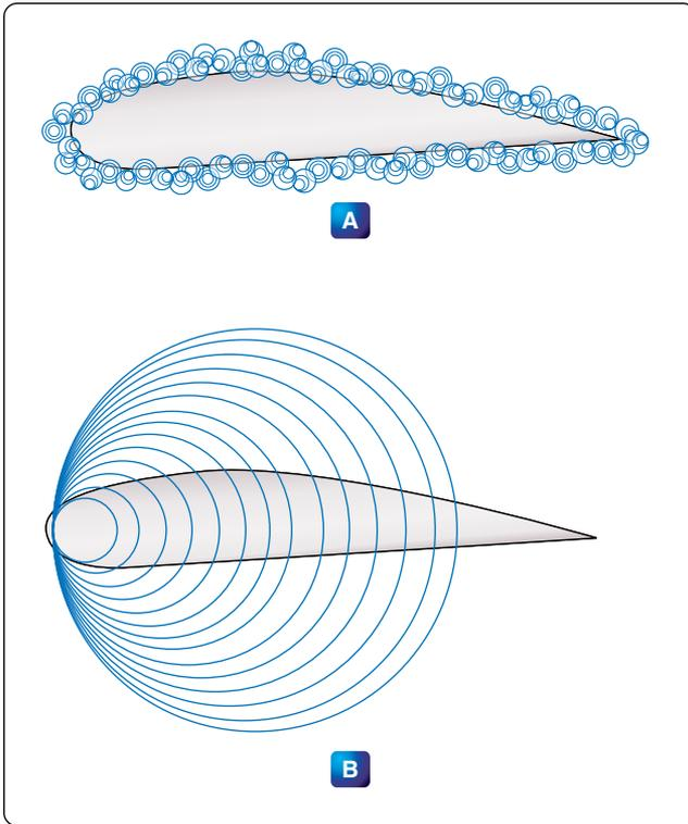
Figure 5-76. Sound energy in subsonic and supersonic flight.
