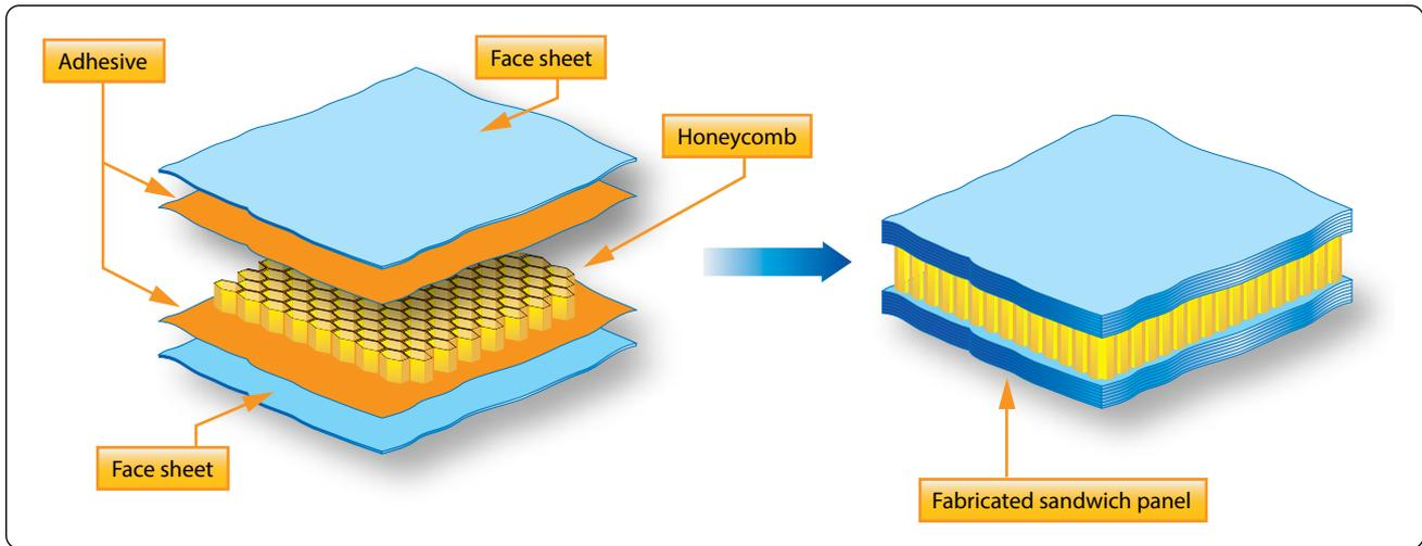
**Figure 7-14.** Sandwich structure.
