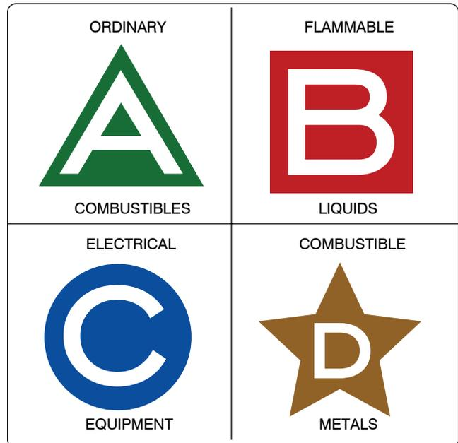
Figure 1-8. Identification of fire extinguisher type location.
