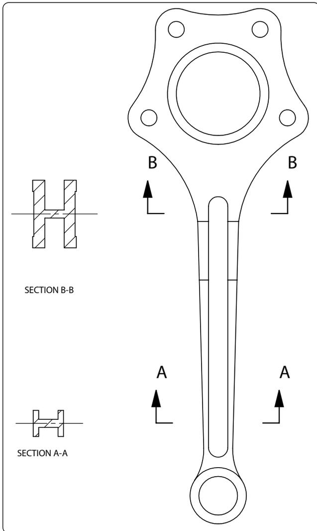
**Figure 4-9.** *Removed sections.*
