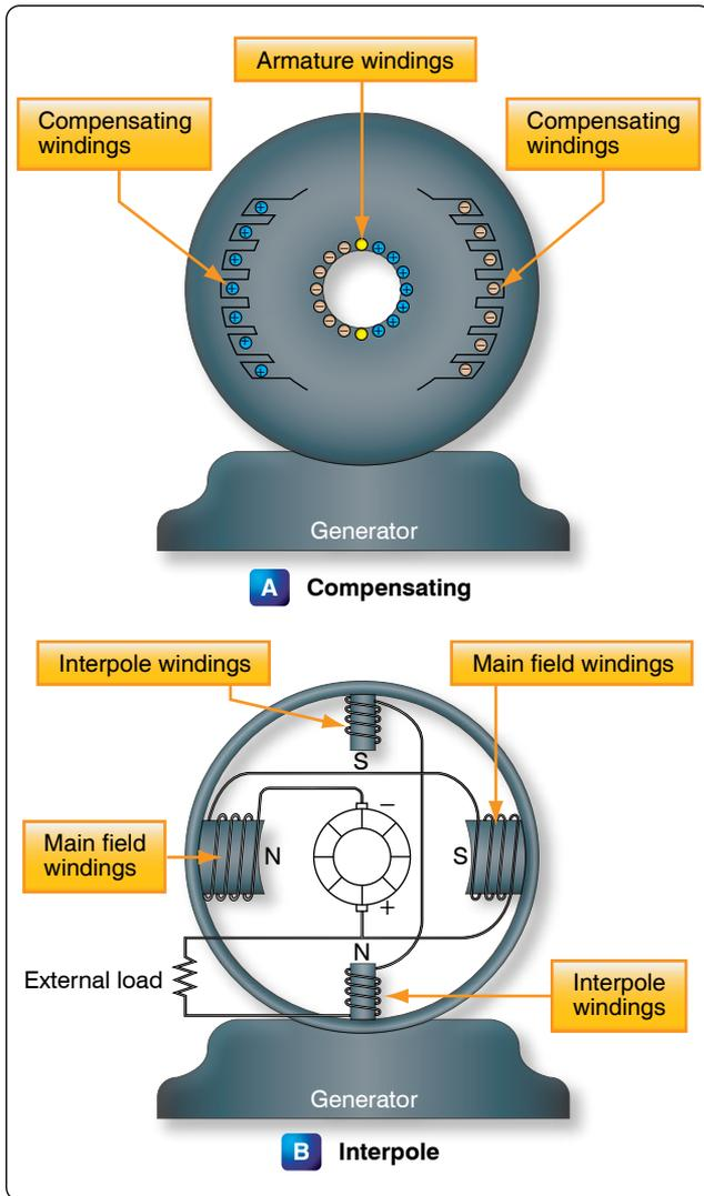
**Figure 12-284.** Simple two-pole generator with two interpoles.
