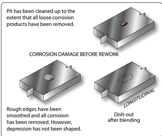
Figure 8-24. Blend of corrosion as a single depression.
