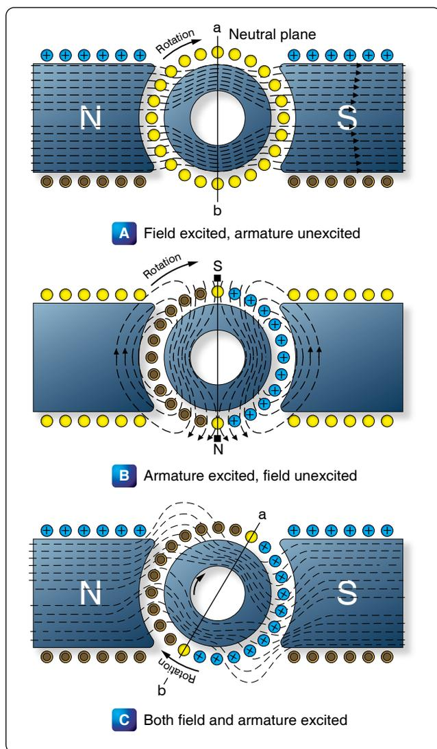
Figure 12-283. Armature reaction.
