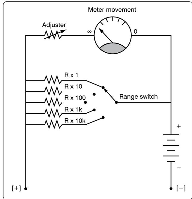
Figure 12-157. Multirange ohmmeter.
