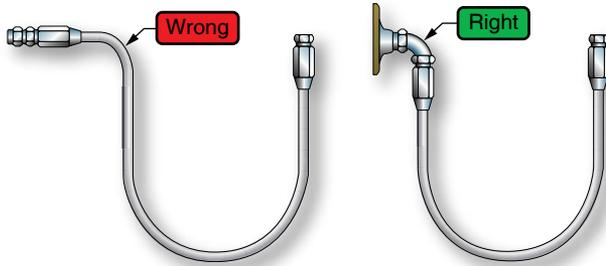
3. Relieve sharp bends, avoid strain or hose collapse, and make cleaner installations by using Aeroquip elbows or other adapter fittings. Provide as large a bend radius as possible. Never use less than the recommended minimum bend radius specified for the hose.
