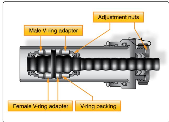
**Figure 7-17.** V-ring installation.
