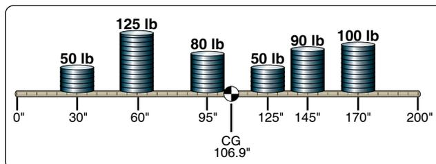
**Figure 6-6.** Center of gravity for weights on a plank with datum at one end.
