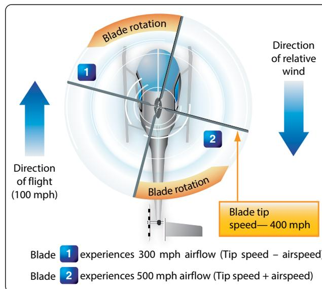
Figure 5-94. Dissymmetry of lift for rotor blades.
