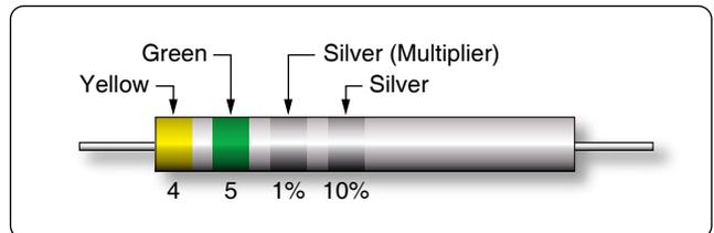
Figure 12-56. Resistor with a silver third band.
