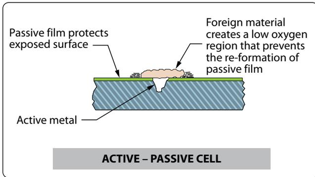
Figure 8-13. Active-passive cell.
