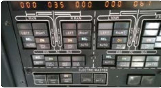
Figure 12-78. Lighted pushbutton switches.
