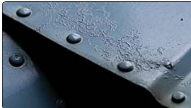
**Figure 8-8.** *Filiform corrosion.*
