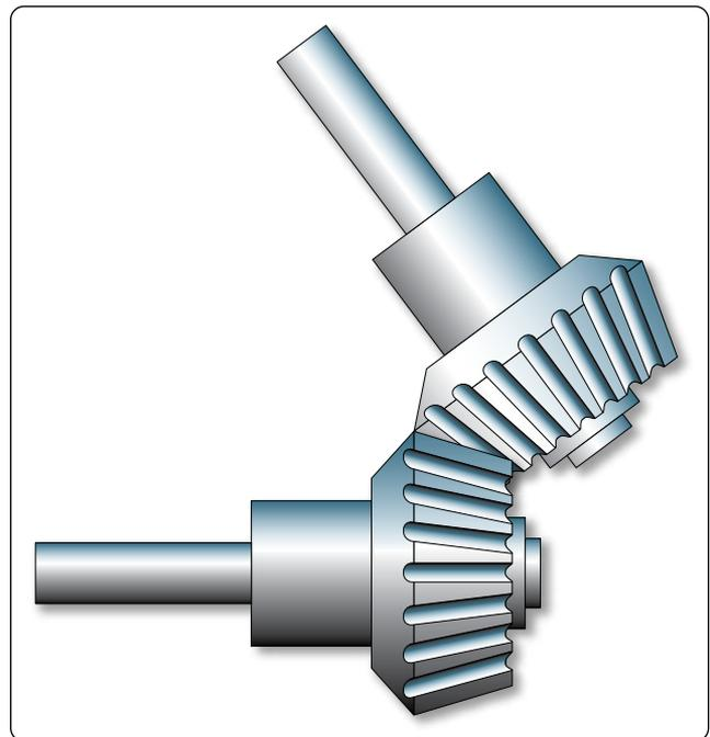
**Figure 5-14.** *Bevel gears.*
