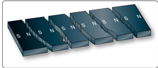
**Figure 12-22.** *Magnetic poles in a broken magnet.*
