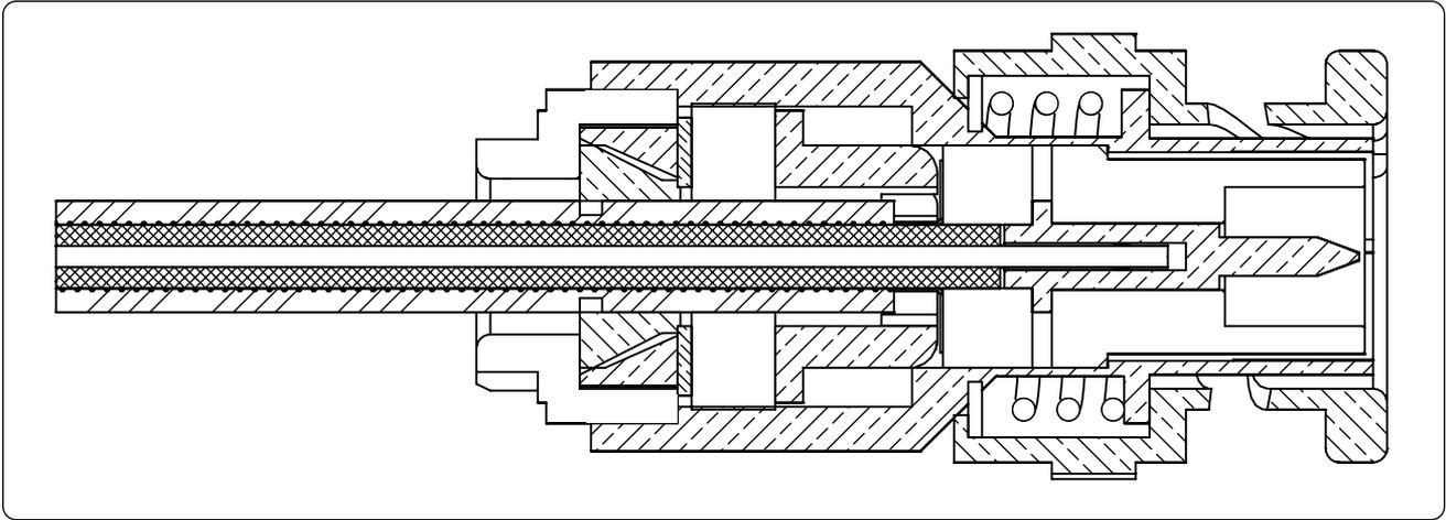
**Figure 4-6.** Sectional view of a cable connector.
