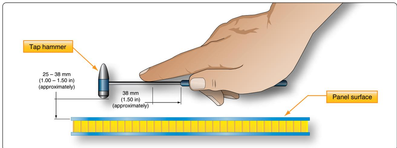
Figure 10-37. Tap testing using hammer.
