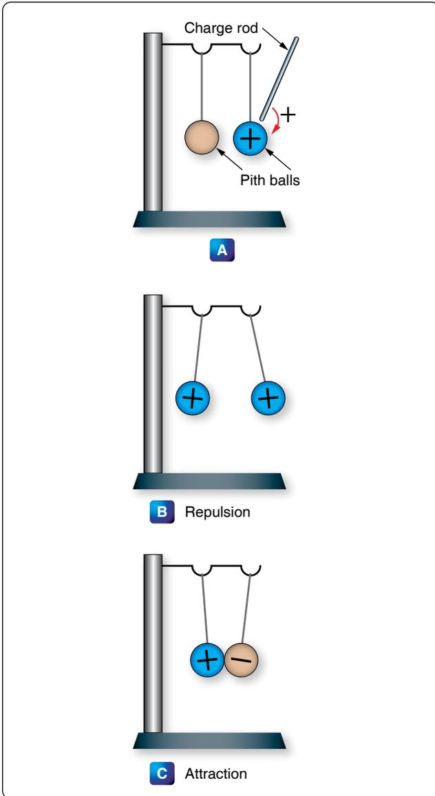
Figure 12-6. Reaction of like and unlike charges.
