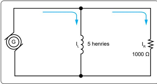
**Figure 12-138.** AC parallel circuit containing inductance and resistance.
