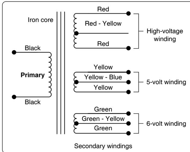
Figure 12-146. Schematic symbol for an iron-core power transformer.
