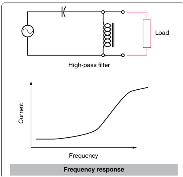
Figure 12-235. High-pass filter.
