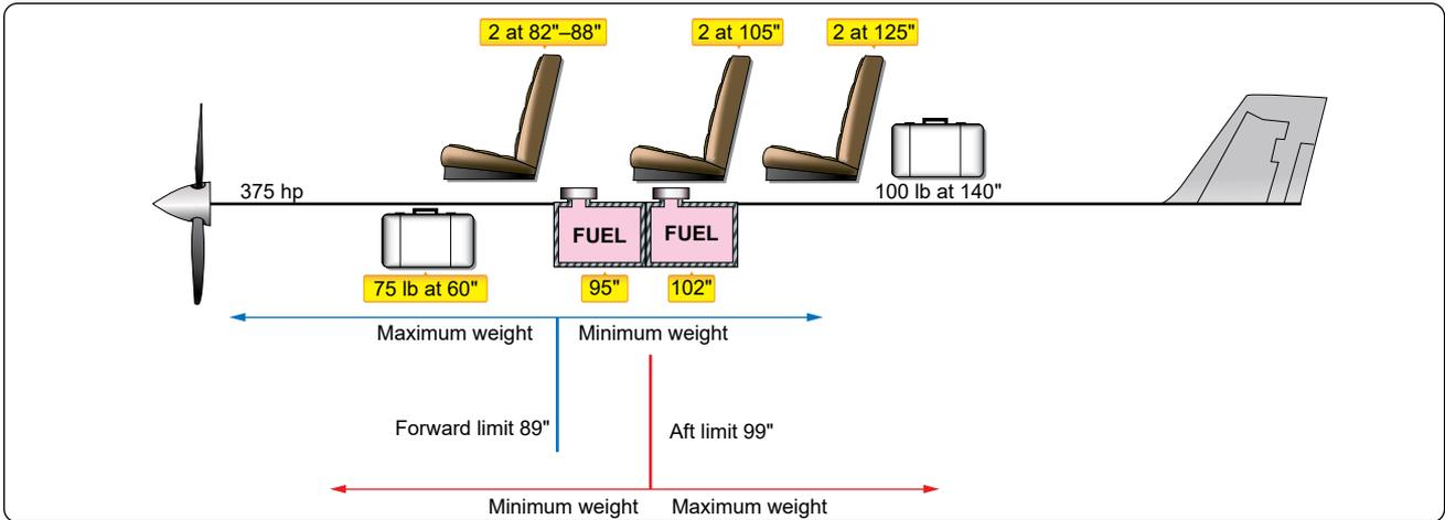
Figure 6-36. Example airplane for extreme condition checks.
