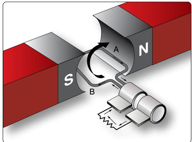
**Figure 12-271.** *Inducing maximum voltage in the opposite direction.*
