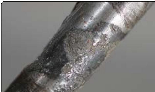
Figure 8-10. Dissimilar metal corrosion.
