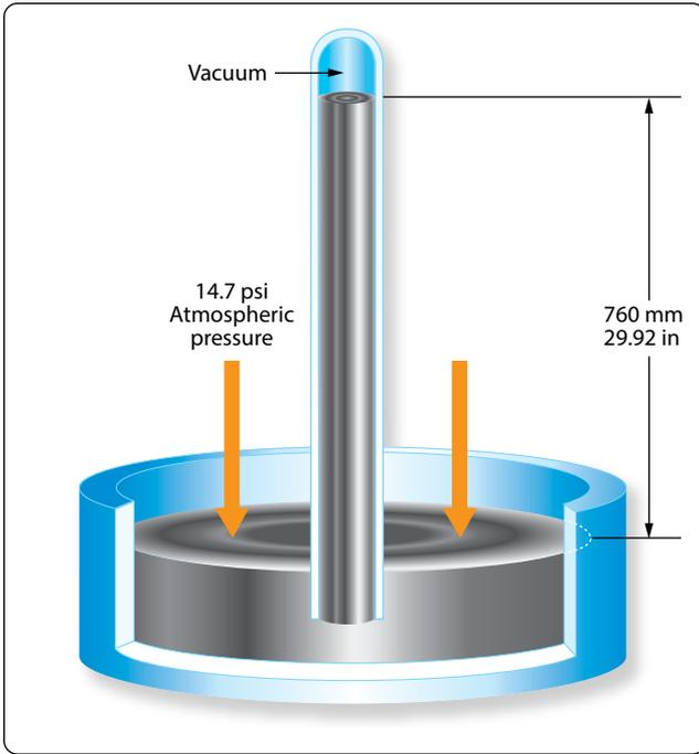
Figure 5-33. Atmospheric pressure as inches of mercury.
