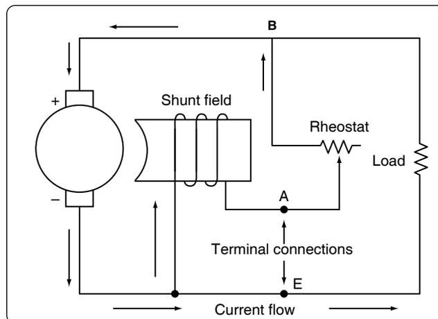
**Figure 12-327.** Regulation of generator voltage by field rheostat.
