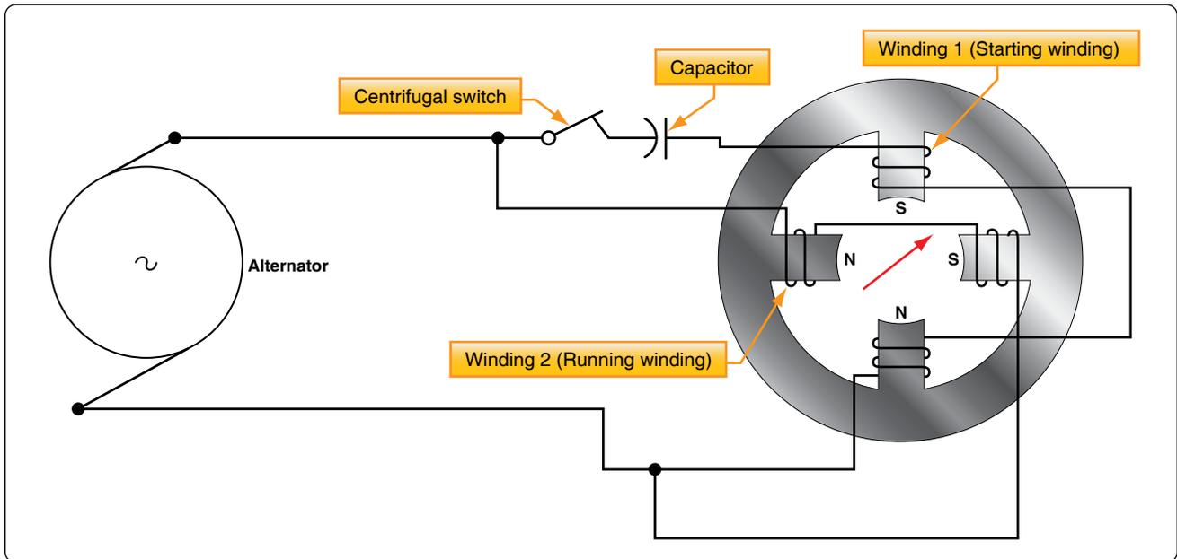
Figure 12-311. Single-phase motor with capacitor starting winding.
