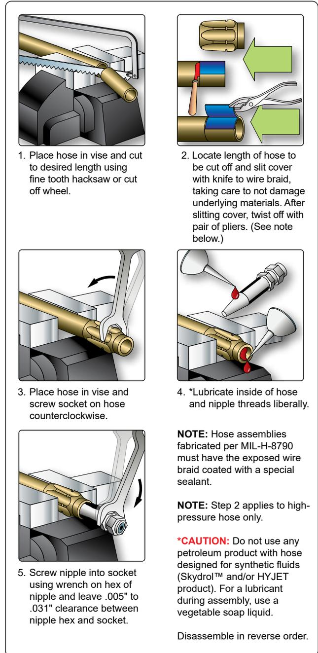
Figure 9-35. Assembly of MS fitting to flexible hose.
