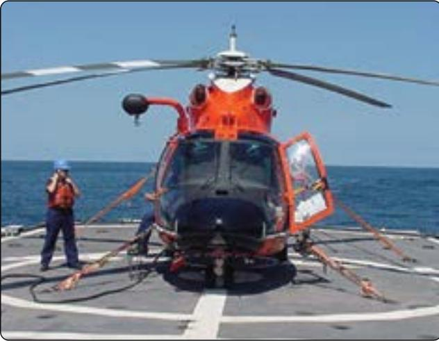
**Figure 1-13.** Example of mooring of a helicopter.
