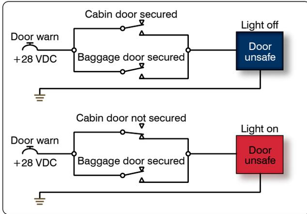
Figure 12-259. Simplified circuit that illustrates OR logic.
