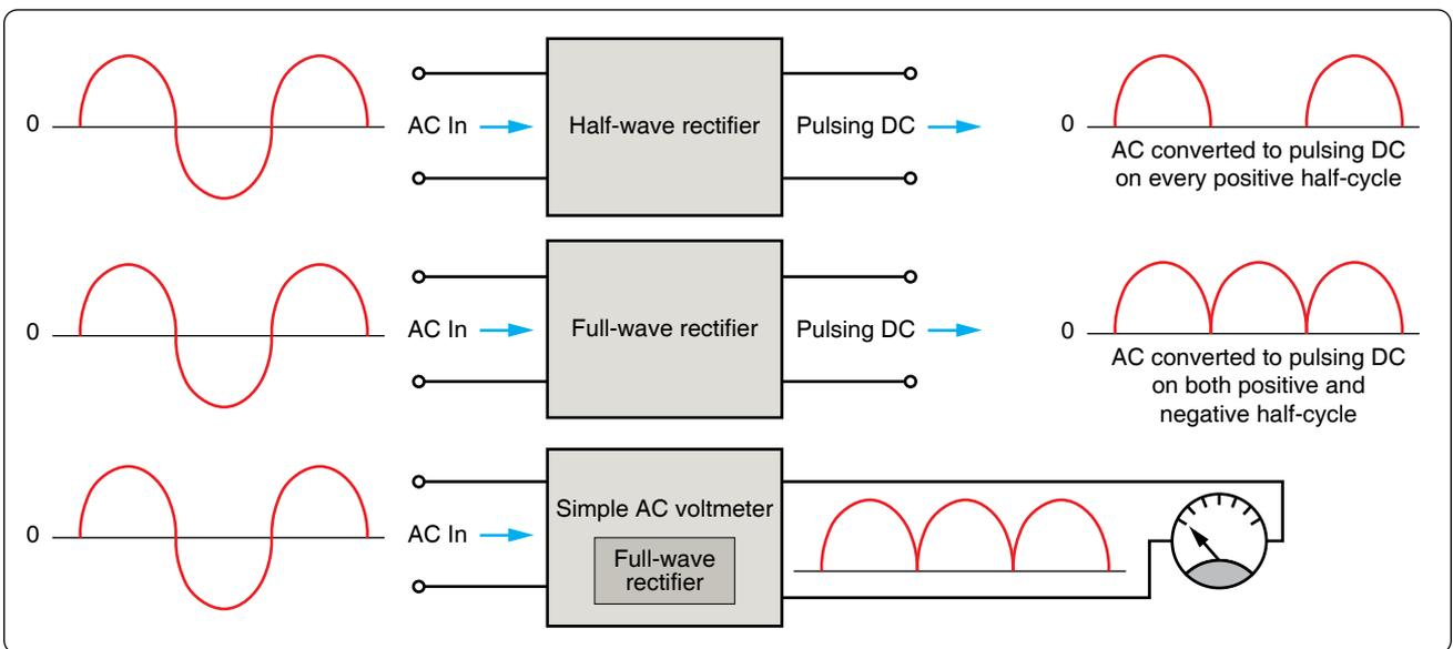
Figure 12-159. Simplified block diagram of AC meter.
