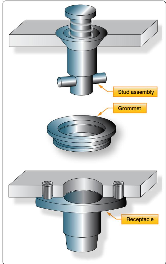
Figure 7-60. Camloc fastener.
