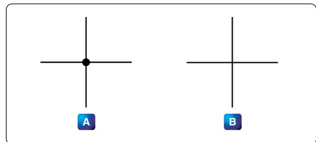
Figure 12-46. Connected wires.
