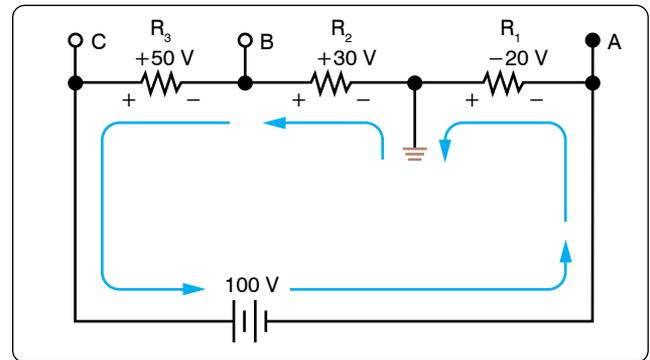
Figure 12-92. Current flow through a voltage divider.
