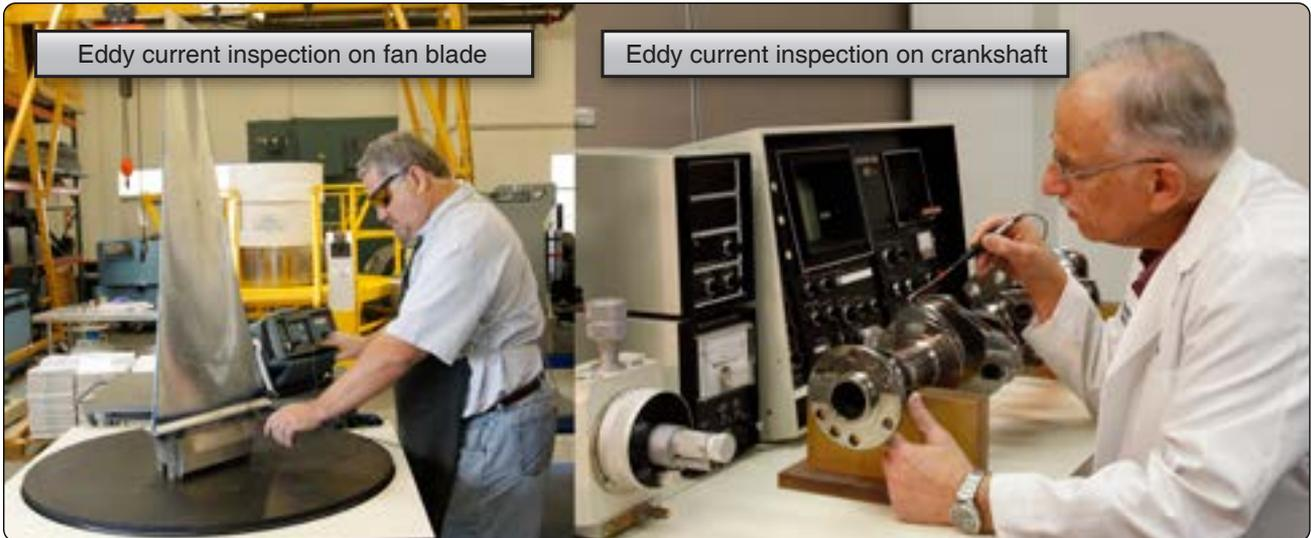
Figure 10-10. Eddy current inspection.
