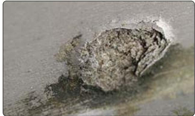
Figure 8-15. Exfoliation corrosion.
