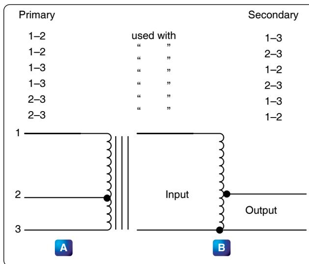
Figure 12-148. Autotransformers.
