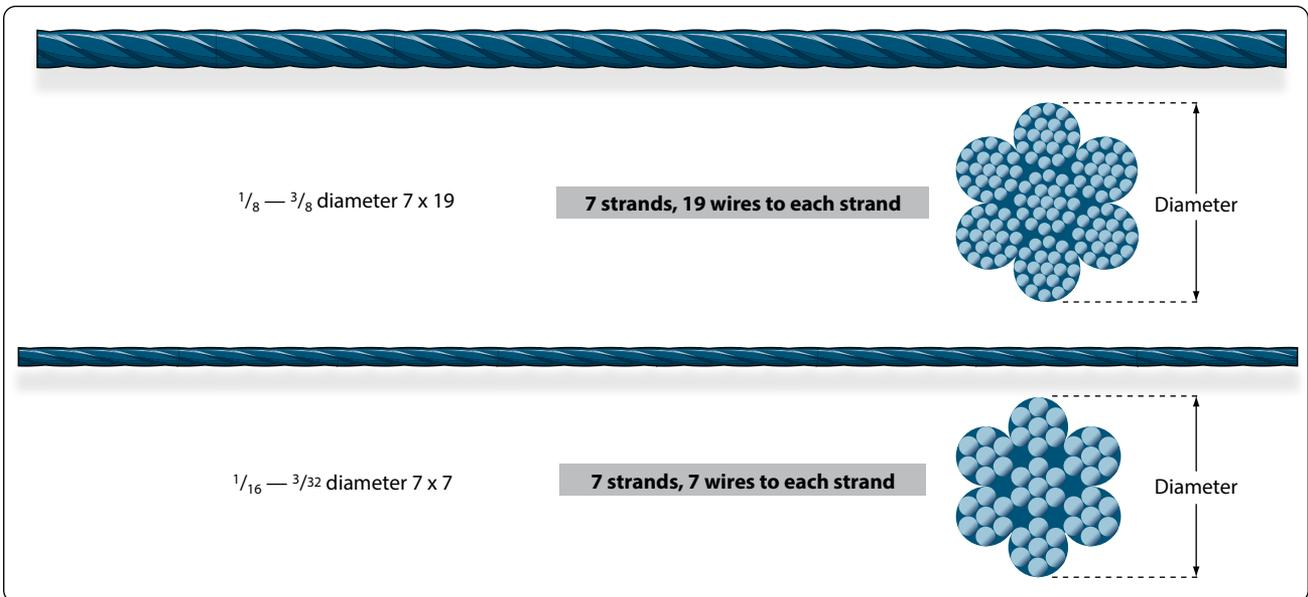
Figure 7-68. Cable cross-sections.
