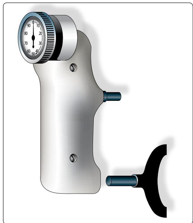
Figure 7-12. Barcol portable hardness tester.
