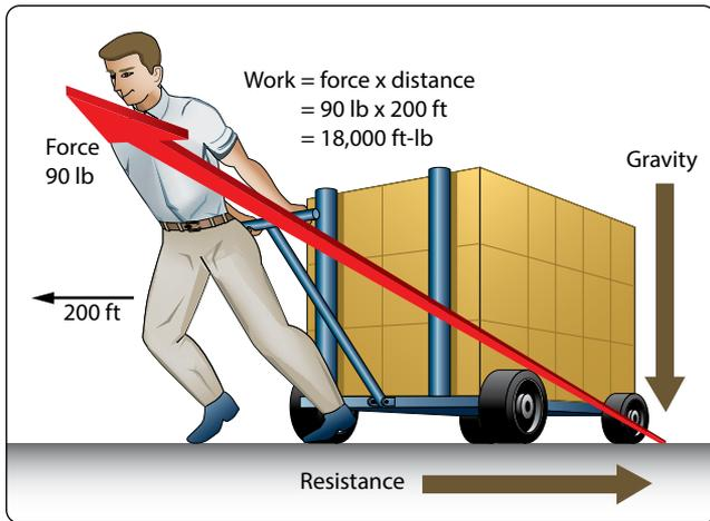
**Figure 5-5.** *The effect of friction on work.*
