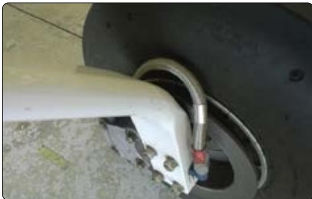
Figure 9-32. Flexible hose with stainless braid.
