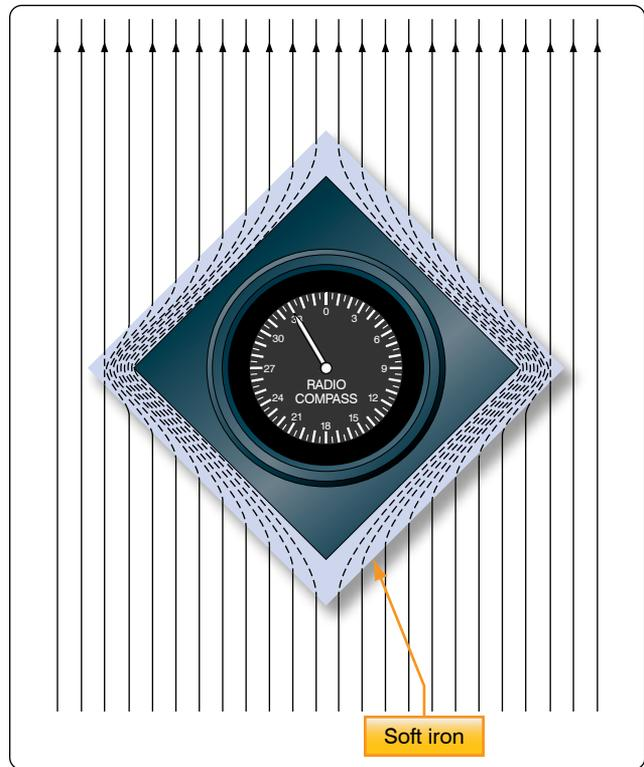
**Figure 12-23.** *Magnetic shield.*
