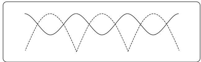
Figure 12-231. Output of an inductor filter rectifier.
