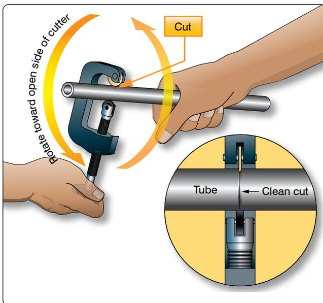
Figure 9-2. Tube cutting.
