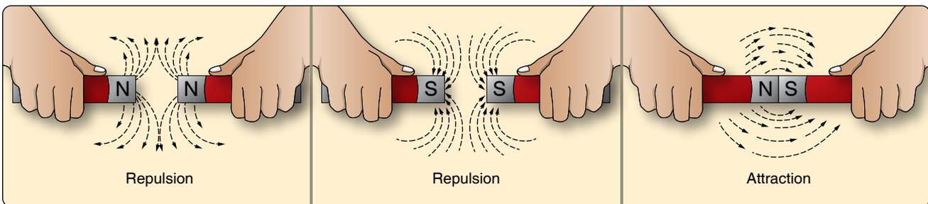
**Figure 12-21.** *Repulsion and attraction of magnet poles.*
