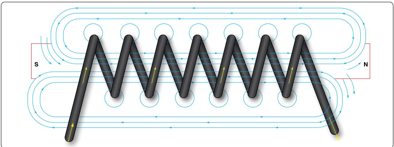
**Figure 12-34.** *Electromagnet.*
