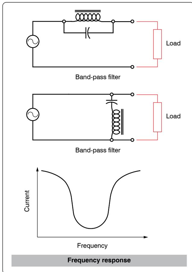
Figure 12-237. Band-stop filter.
