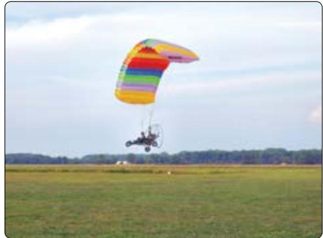
**Figure 5-102.** *Powered parachute with the wing inflated.*
