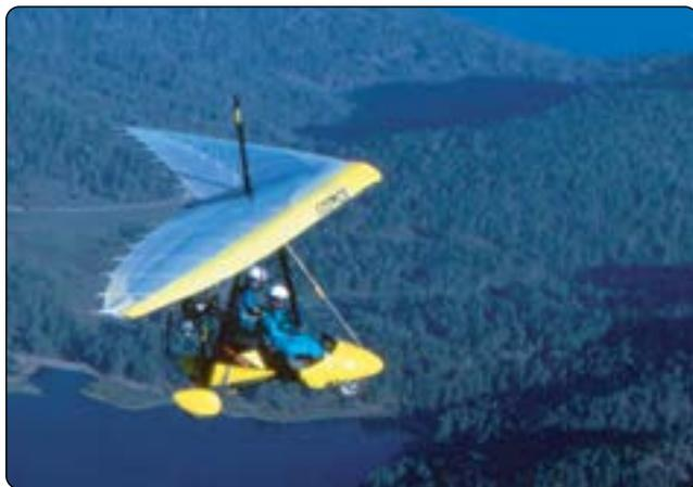
**Figure 5-97.** *Weight-shift control aircraft in level flight.*
