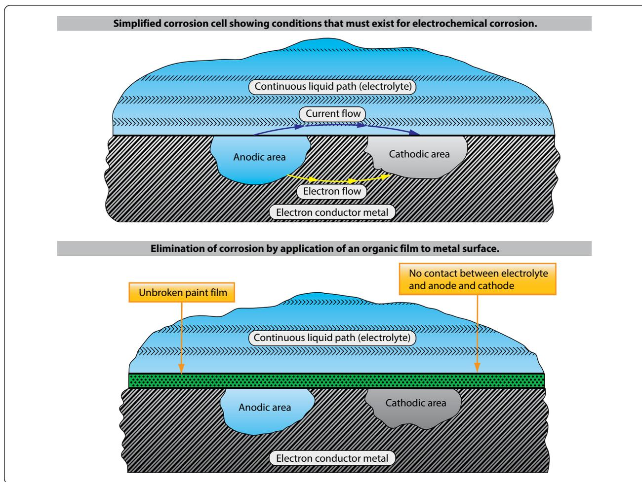
Figure 8-5. Electrochemical attack.
