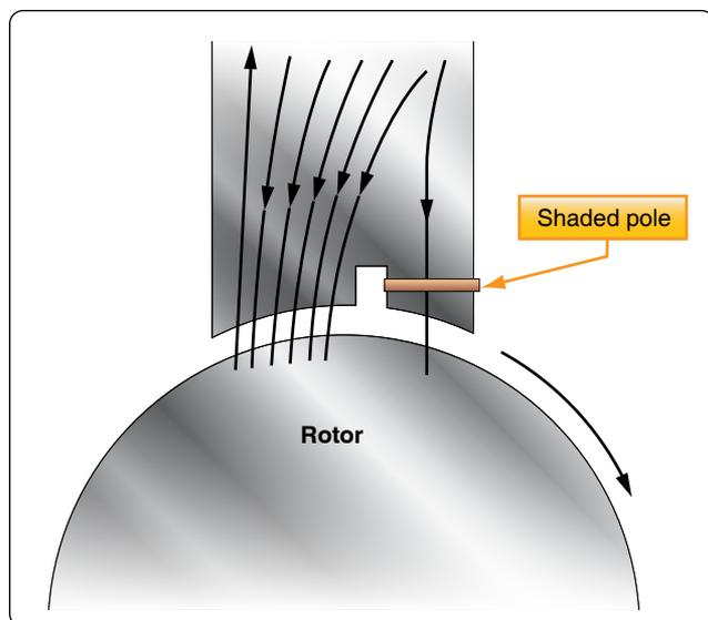
**Figure 12-310.** Diagram of a shaded pole motor.
