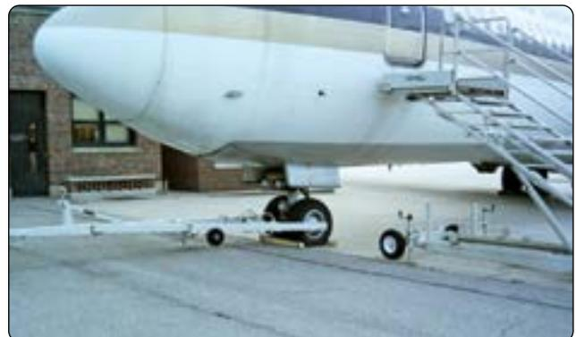
**Figure 1-20.** Example of a tow bar.
