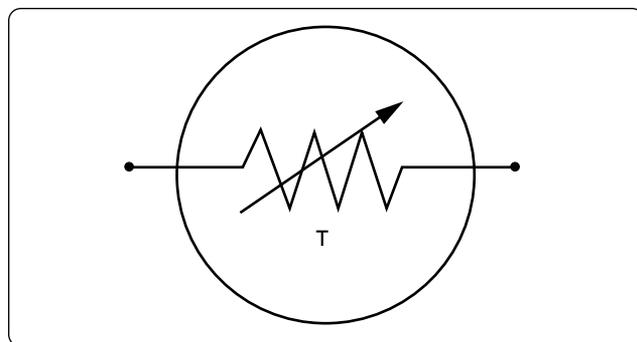
Figure 12-65. Schematic symbol for thermistor.
