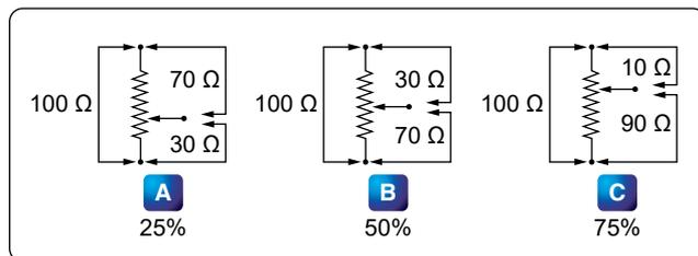
Figure 12-64. Tapered potentiometer.
