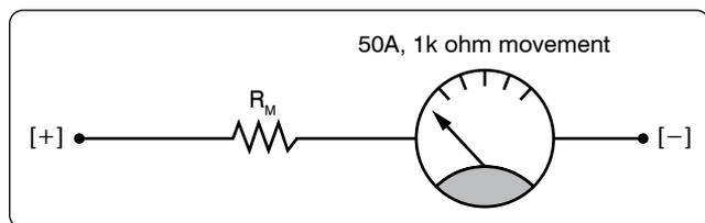
Figure 12-152. Basic voltmeter.
