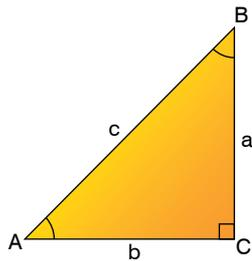
$$\text{Sine (sin) of angle A} = \frac{\text{opposite side (side a)}}{\text{hypotenuse (side c)}}$$
