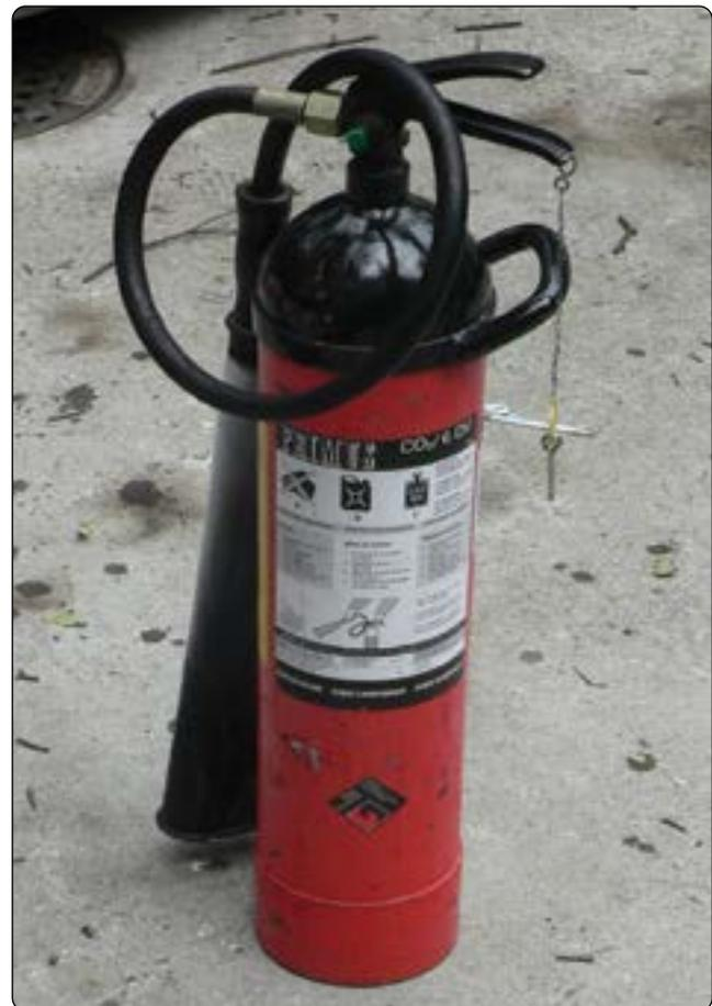
**Figure 1-4.** Carbon dioxide fire extinguisher.
