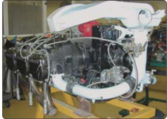
**Figure 5-29.** Aircraft piston engine cooled by convection.
