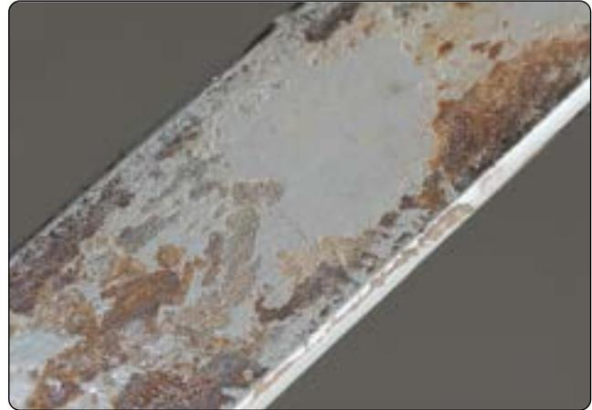
**Figure 8-17.** *Fretting corrosion.*
