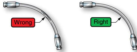
2. Observe linear stripe. The hose must not be twisted. High pressures applied to a twisted hose may cause failure or loosen the nut.
