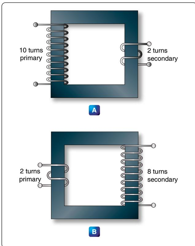
Figure 12-144. A step-down and a step-up transformer.
