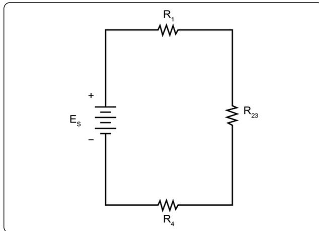
Figure 12-101. Equivalent circuit with three series connected resistors.
