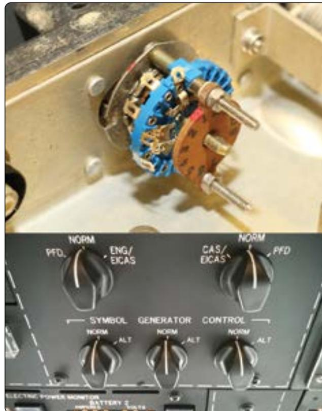
Figure 12-77. Rotary switches.
