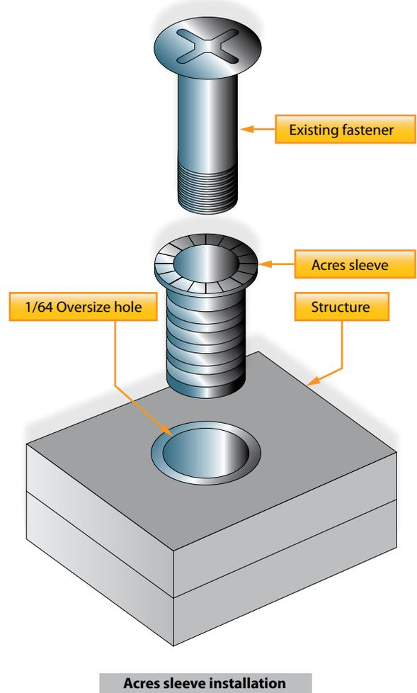
Figure 7-67. Acres sleeve identification, installation, and breakoff procedure.
