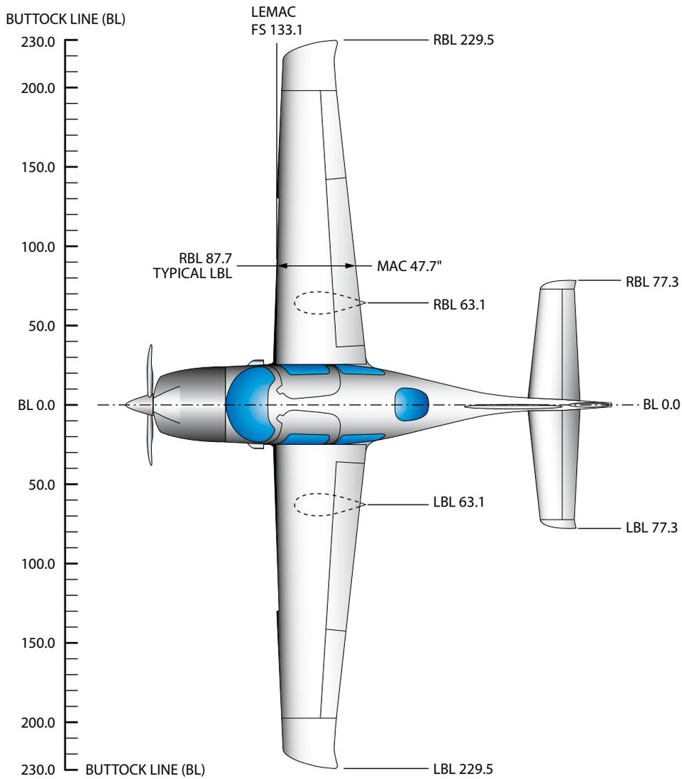
Figure 4-10. Station numbers and location identification on aircraft.
