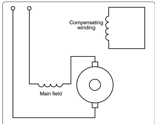
Figure 12-315. Inductively compensated armature of AC series motor.
