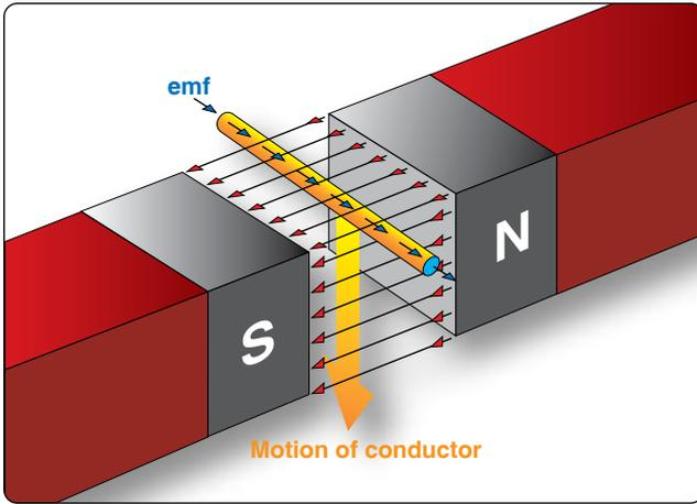
Figure 12-105. Inducing an emf in a conductor.
