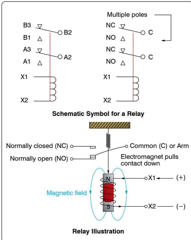
Figure 12-80. Basic relay.
