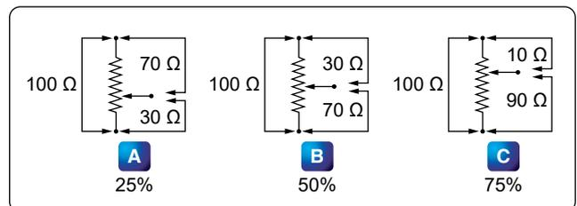
Figure 12-63. Linear potentiometer schematic.
