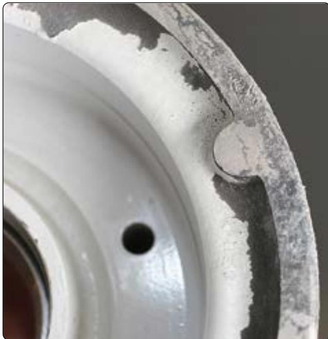
Figure 8-29. Magnesium corrosion.
