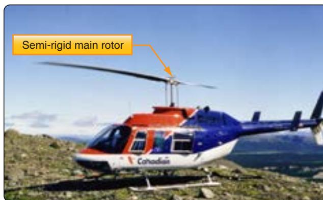
Figure 5-84. Bell Jet Ranger with semi-rigid main rotor.
