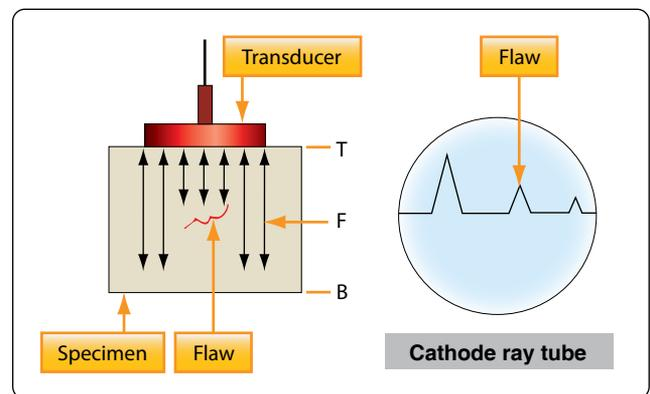
Figure 10-21. Pulse-echo display in relationship to flaw detection.
