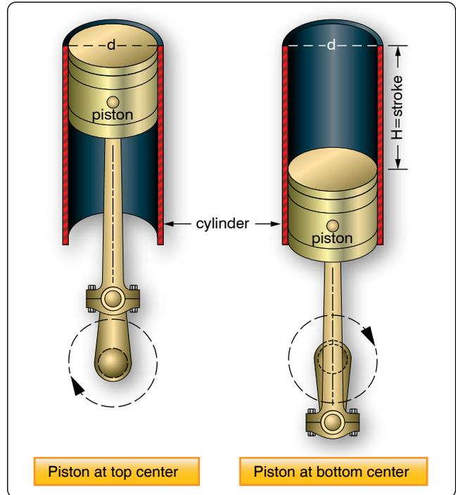
Figure 3-27. Cylinder displacement.
