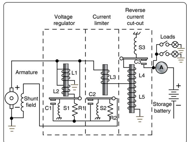
Figure 12-330. Three unit regulator for variable speed generators.
