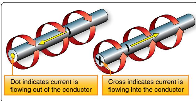
**Figure 12-30.** *Direction of current flow in a conductor.*
