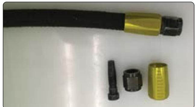
Figure 9-36. MS-type end fitting.
