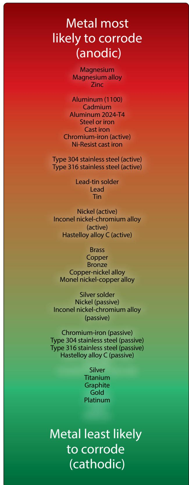
**Figure 8-6.** The galvanic series of metals and alloys.
