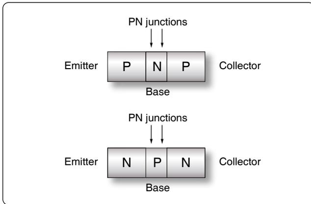
**Figure 12-220.** *Transistor.*
