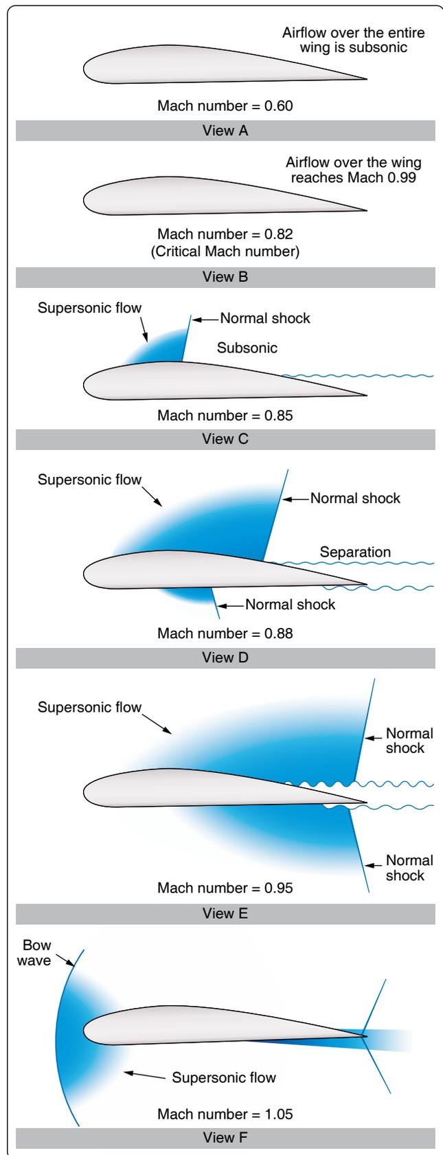
**Figure 5-79.** Airflow with progressively greater Mach numbers.
