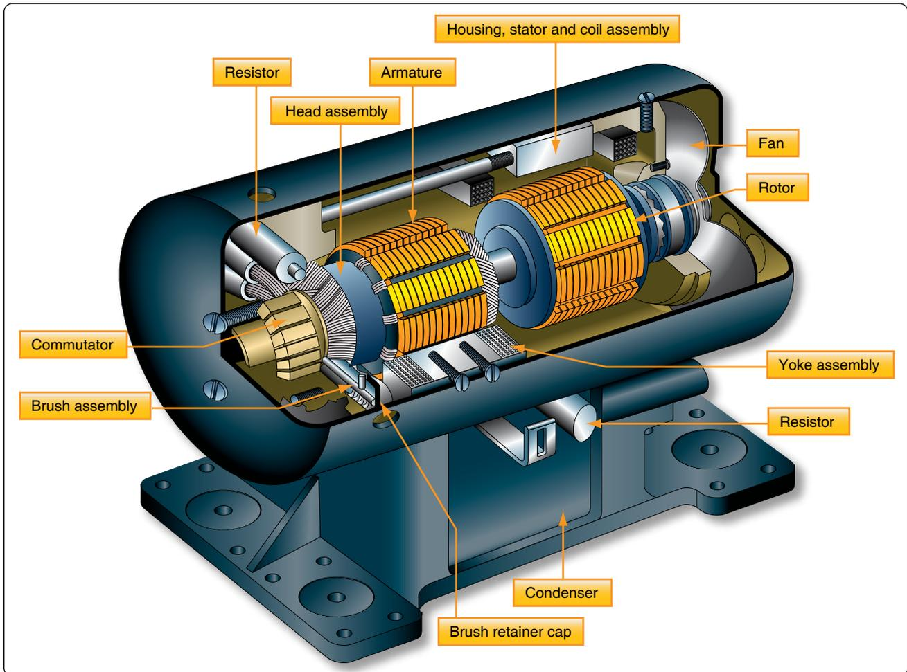
**Figure 12-204.** Cutaway view of inductor-type rotary inverter.
