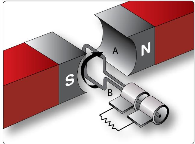
**Figure 12-270.** *Inducing minimum voltage in an elementary generator.*
