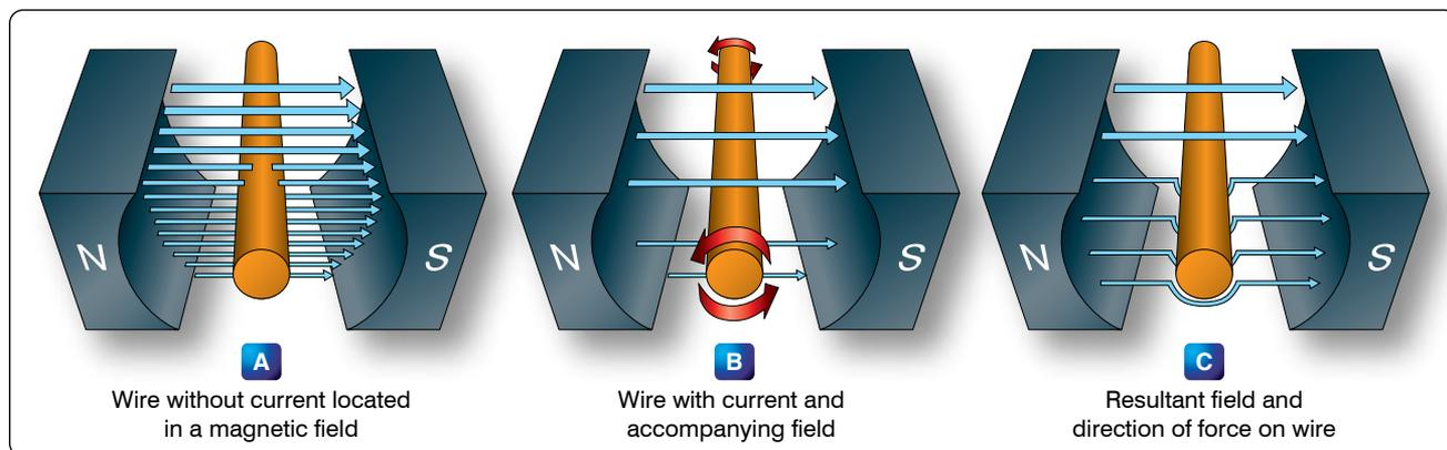
Figure 12-291. Force on a current carrying wire.
