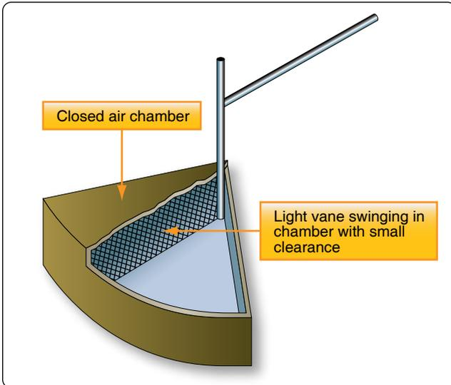
Figure 12-150. Air damping.
