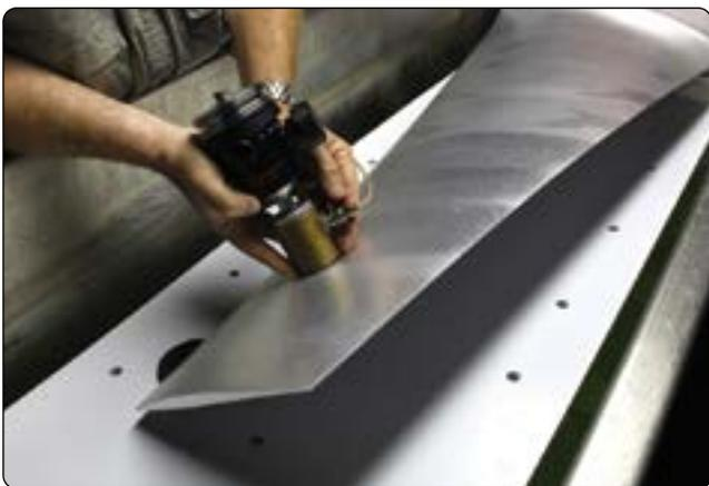
**Figure 10-25.** Ultrasonic inspection of a composite structure.
