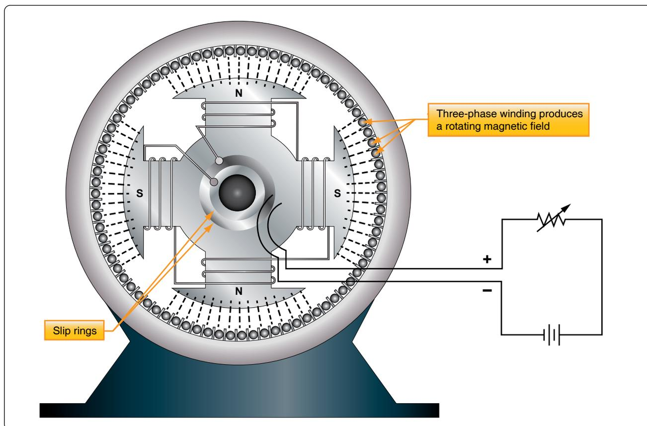
Figure 12-313. Synchronous motor.
