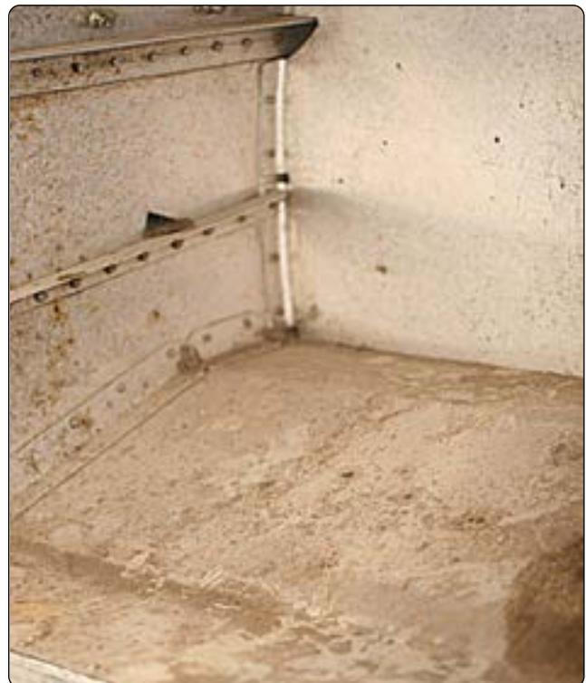
Figure 8-4. Direct chemical attack in a battery compartment.
