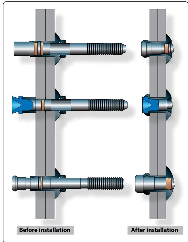
Figure 7-43. Self-plugging (mechanical lock) rivets.
