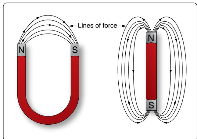
Figure 12-15. Magnetic field around magnets.
