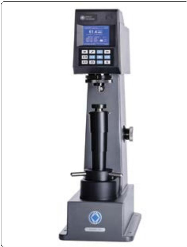
Figure 10-5. Rockwell C Hardness Tester.
