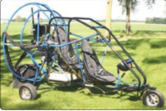
**Figure 5-103.** *Two seat powered parachute.*
