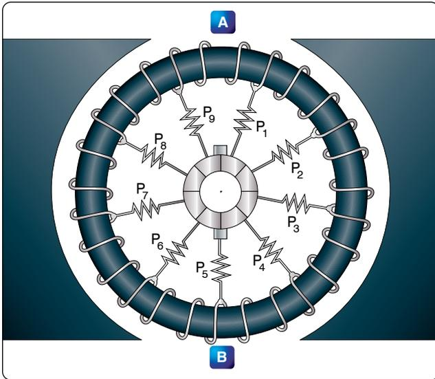
**Figure 12-316.** Preventive coils in AC series motor.
