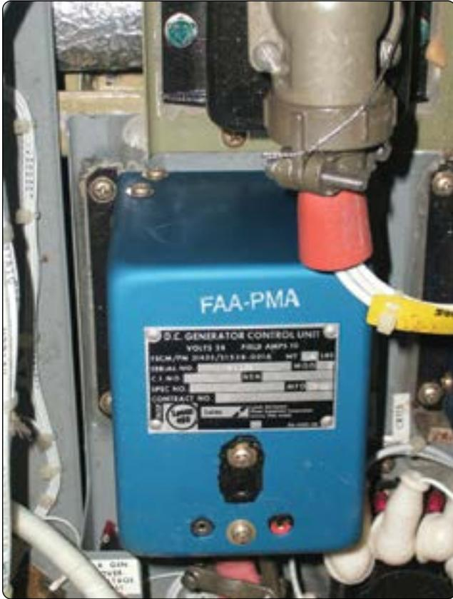
**Figure 12-332.** Generator Control Unit (GCU).
