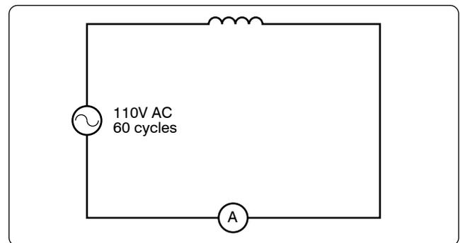
Figure 12-130. AC circuit containing inductance.
