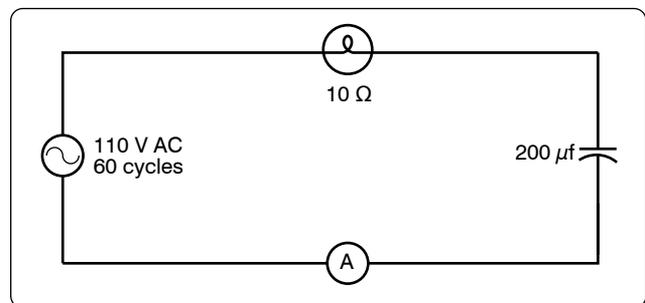
**Figure 12-136.** A circuit containing resistance and capacitance.
