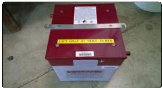
**Figure 12-199.** Sealed battery.
