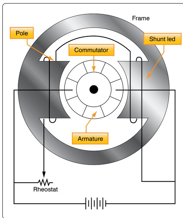
Figure 12-305. Shunt motor with variable speed control.
