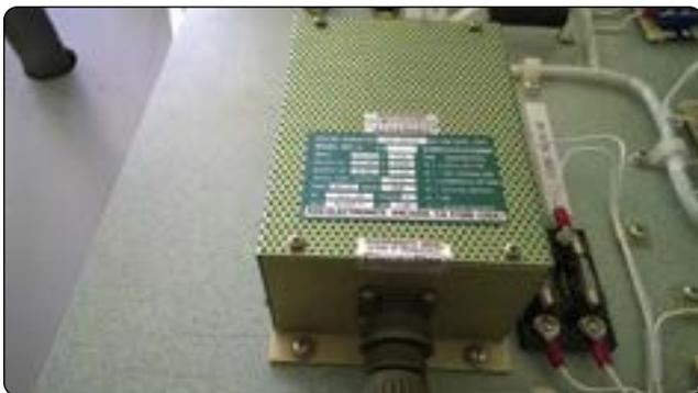
**Figure 12-206.** Static inverter.
