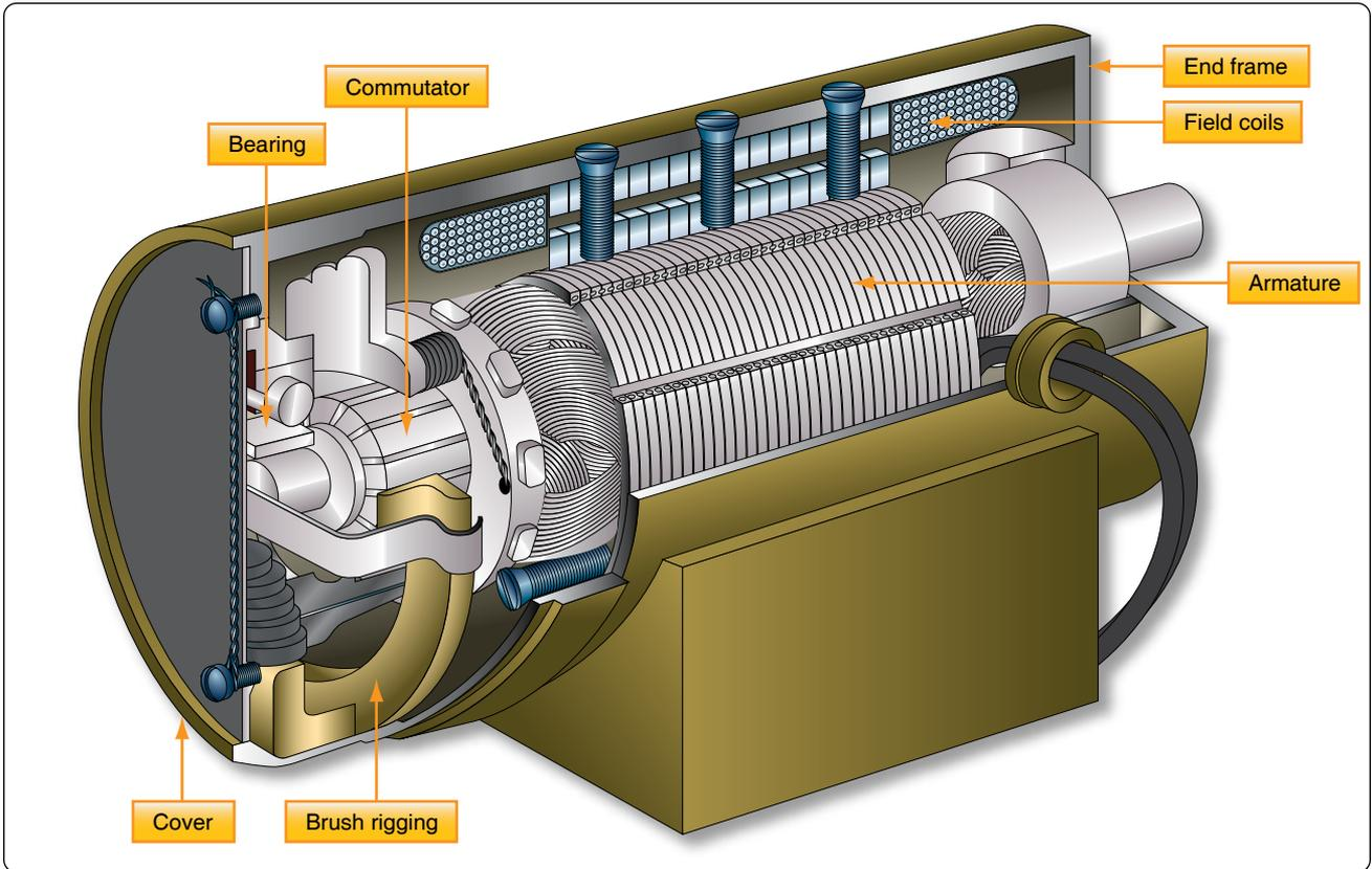
Figure 12-297. Cutaway view of practical DC motor.
