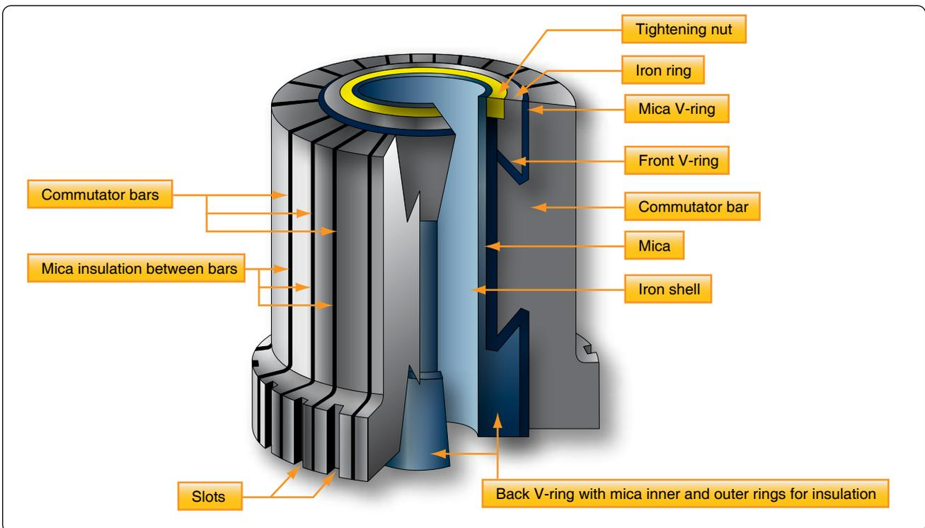
Figure 12-282. Commutator with portion removed to show construction.
