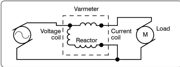
**Figure 12-162.** A varmeter connected in an AC circuit.
