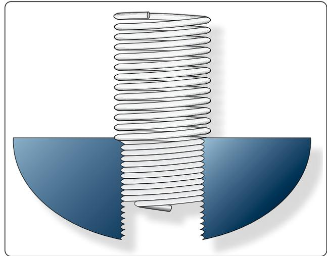
Figure 7-31. Helicoil insert.
