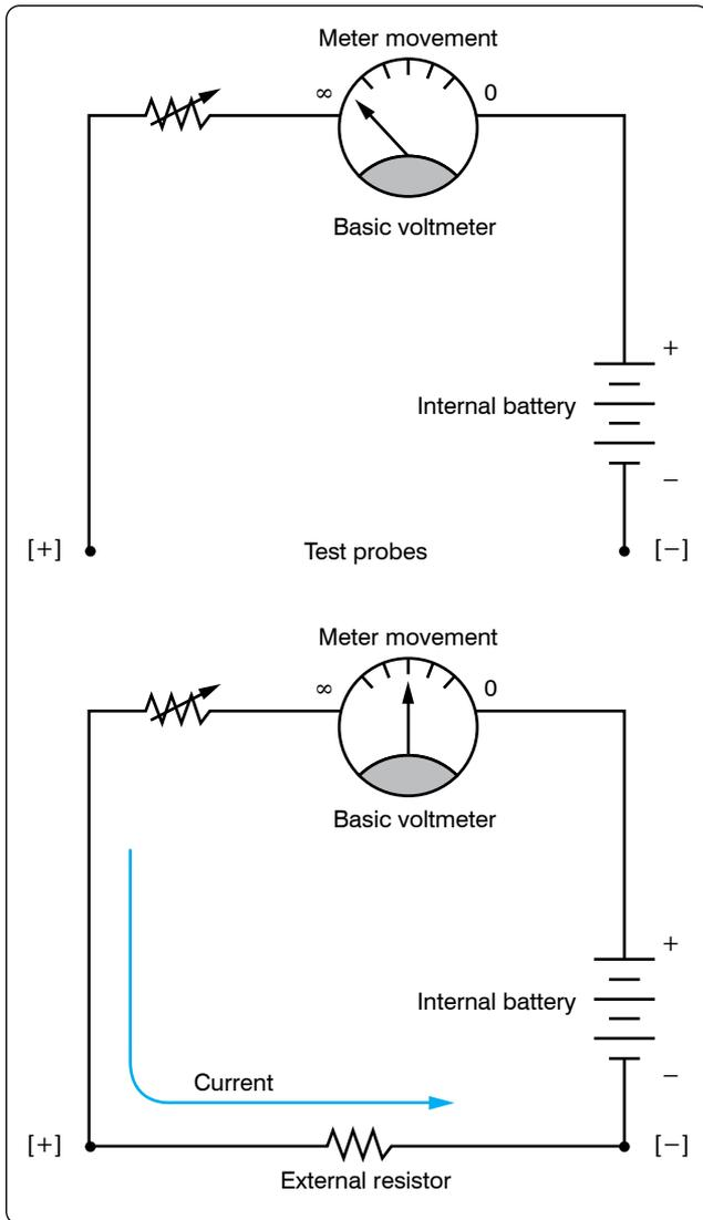
Figure 12-154. Basic ohmmeter.
