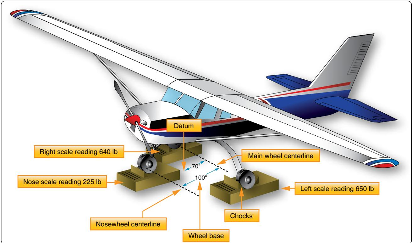
Figure 6-26. Example airplane being weighed. The datum is 70" forward of the wing root leading edge.
