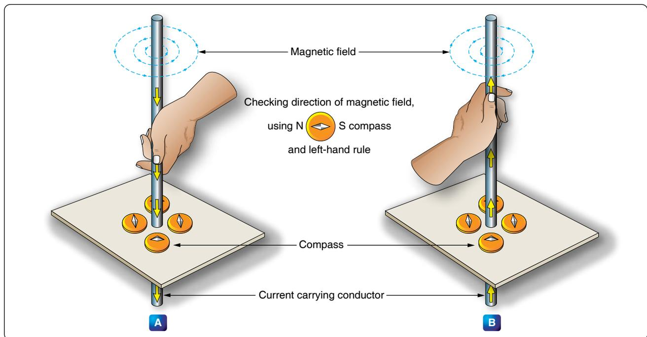
Figure 12-28. Magnetic field around a current-carrying conductor.
