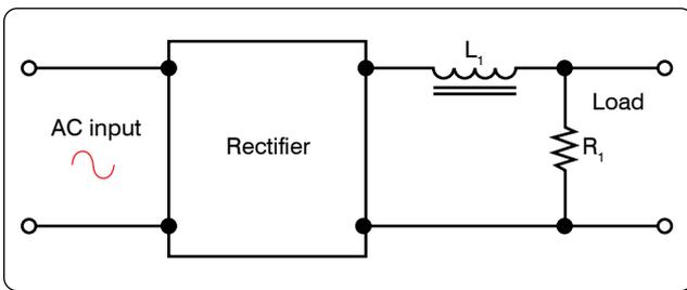
Figure 12-230. An inductor used as a filter.
