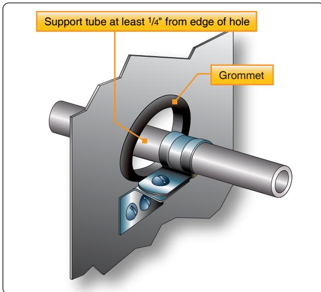
**Figure 9-42.** Rubber-cushioned clamp.
