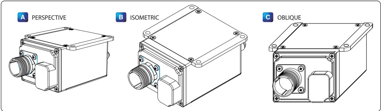
Figure 4-16. (A) Perspective, (B) isometric, and (C) oblique drawings.
