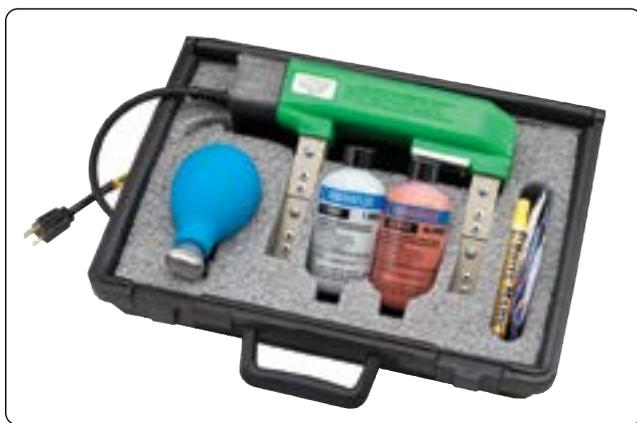
**Figure 10-34.** *Portable magnetic particle inspection equipment.*
