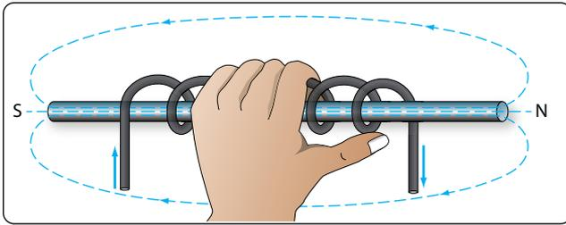
Figure 12-35. Left-hand rule applied to a coil.
