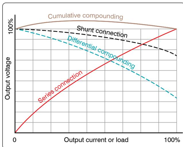
Figure 12-288. Generator characteristics.
