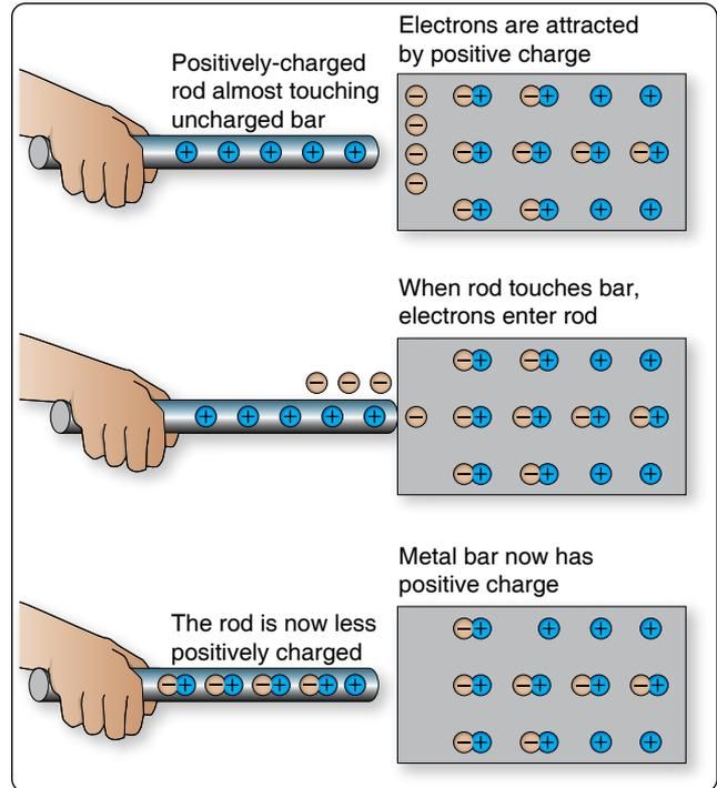
Figure 12-7. Charging by contact.
