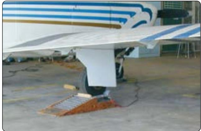
Figure 5-17. Ramp in use with a Mooney M20.
