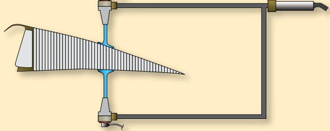
Figure 10-19. Through-transmission and pulse echo indications.
