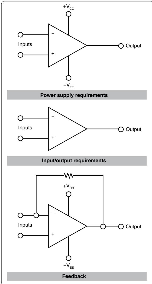
Figure 12-246. Schematic symbol for the operational amplifier.
