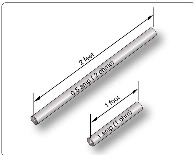
Figure 12-41. Resistance varies with length of conductor.
