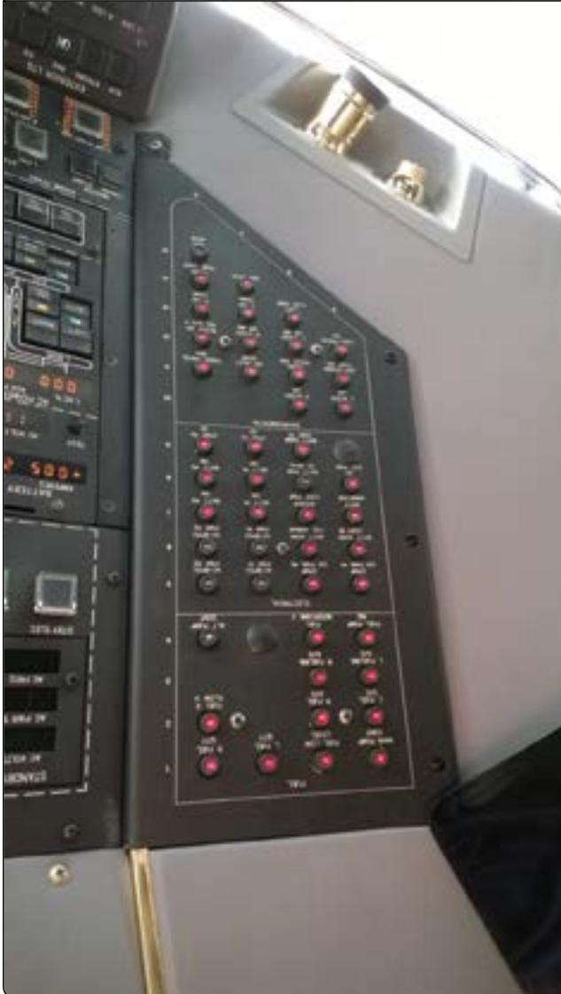
**Figure 12-69.** Circuit breaker assembly for aircraft electrical system.
