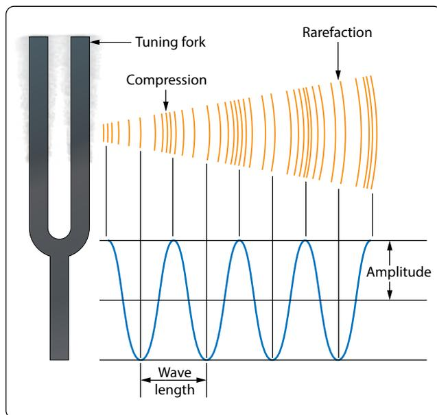
Figure 5-48. Sound propagation by a tuning fork.
