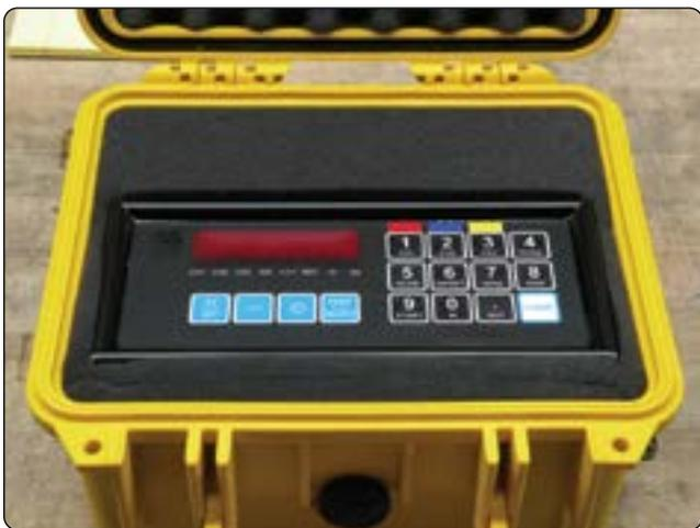
**Figure 6-19.** M2000 platform scale digital indicator.
