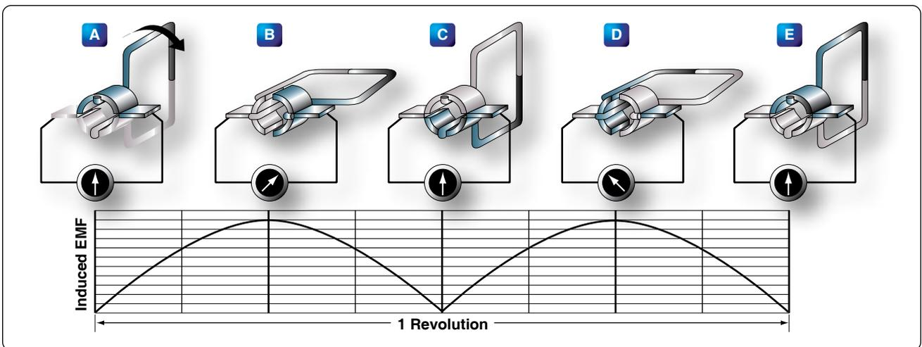
**Figure 12-275.** Operation of a basic DC generator.
