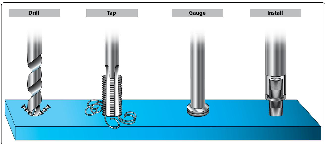
Figure 7-32. Helicoil installation.
