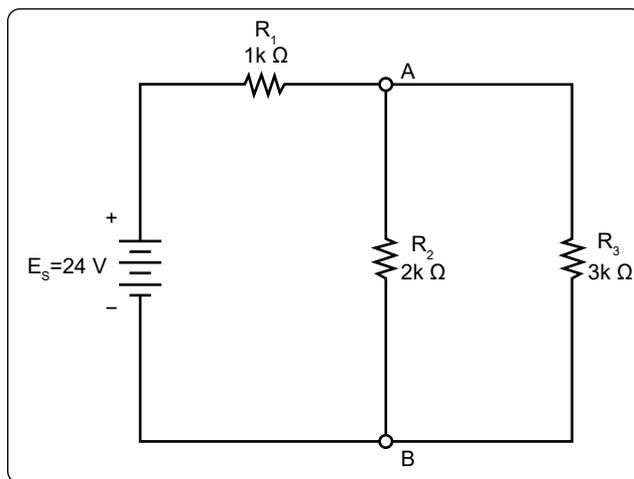
Figure 12-102. Determining total resistance.
