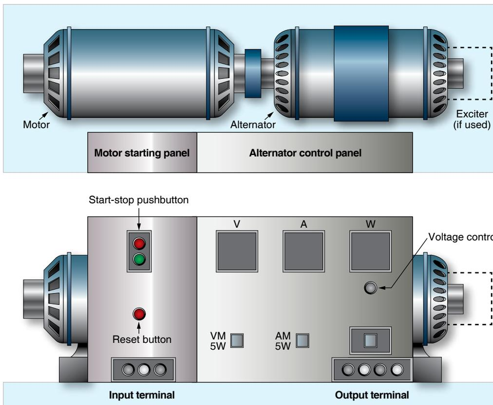
**Figure 12-326.** AC motor generator set for ground testing.
