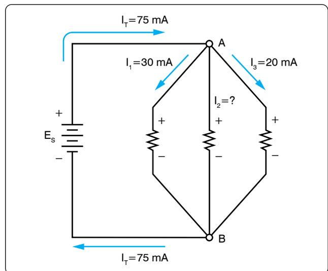
Figure 12-99. Determining an unknown circuit in branch 2.
