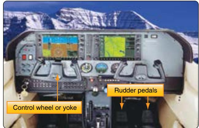
**Figure 5-68.** Cessna 182 control wheel and rudder pedals.
