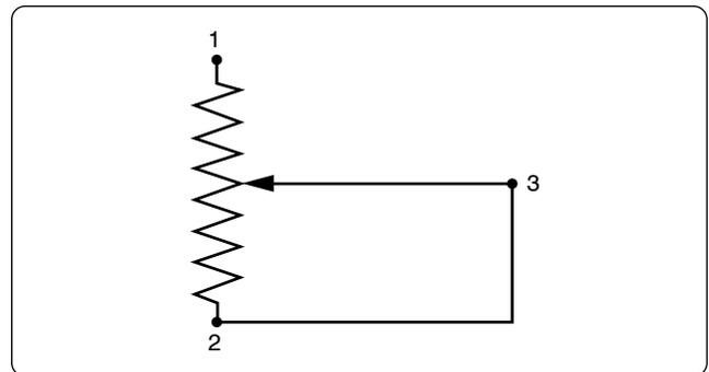
Figure 12-62. Potentiometer wired to function as rheostat.
