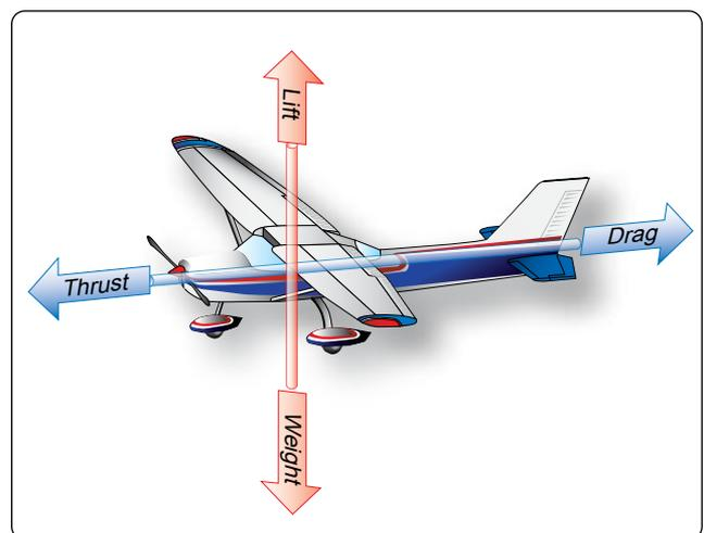
**Figure 5-53.** Four forces acting on an airplane.
