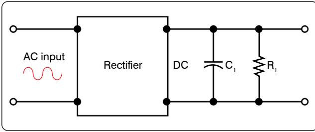
Figure 12-228. A capacitor used as a filter.
