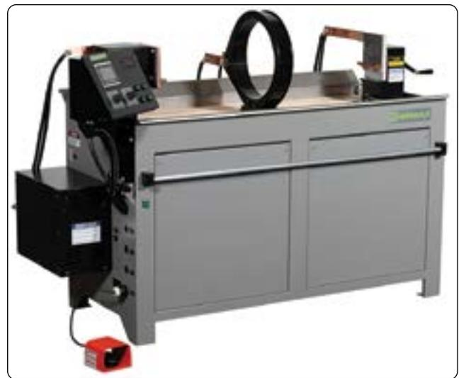
**Figure 10-33.** Fixed general-purpose magnetizing unit.
