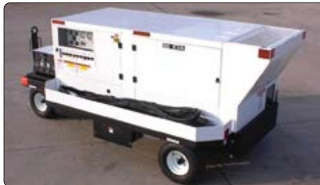
**Figure 1-27.** *A mobile electrical power unit.*
