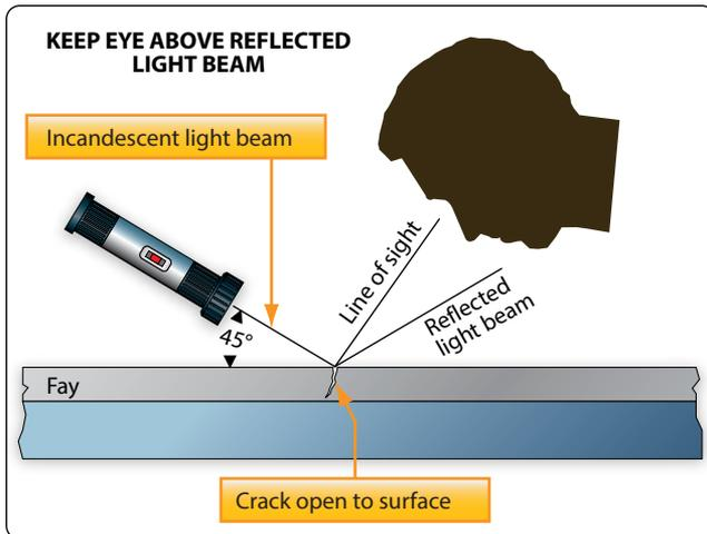
**Figure 10-7.** Using a flashlight to inspect for cracks.
