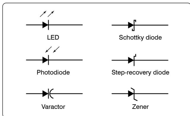
**Figure 12-219.** Schematic symbols for special purpose diodes.
