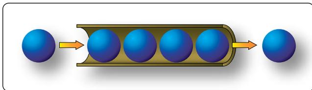
**Figure 12-38.** *Electron movement.*
