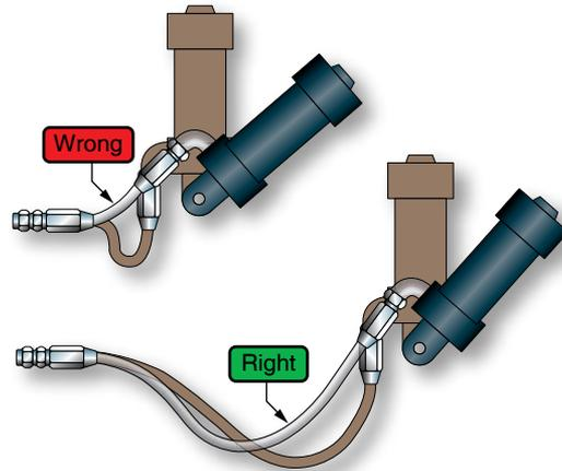
4. Provide additional bend radius when lines are subject to flexing and remember that the metal end fittings are not flexible. Place line support clamps so as not to restrict hose flexing.
