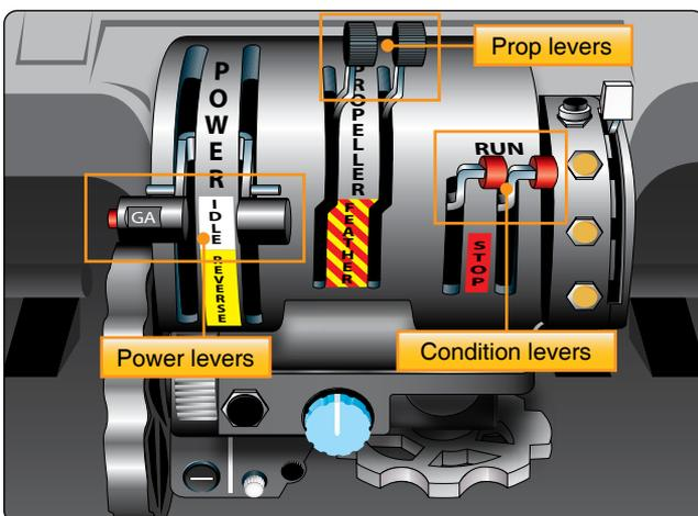
Figure 1-16. Engine controls of a turboprop aircraft.
