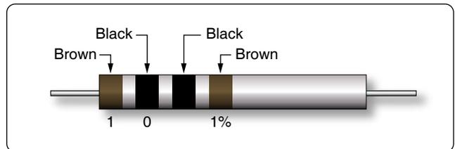
Figure 12-54. Resistor with black third color band.
