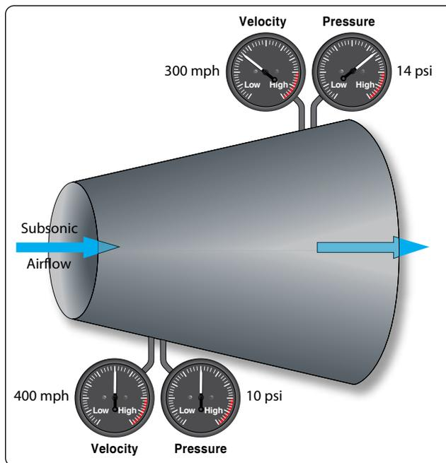
**Figure 5-55.** Bernoulli's principle and a diverging duct.
