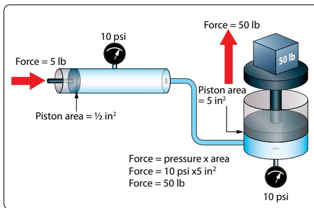
Figure 5-44. Output force created in a hydraulic system.
