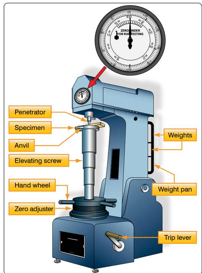
Figure 7-10. Rockwell hardness tester.
