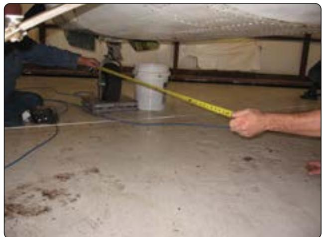
**Figure 6-23.** Measuring the nosewheel arm on an airplane.
