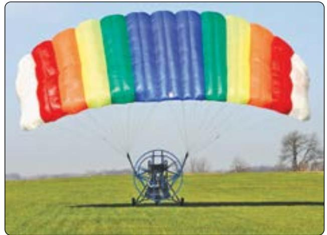
**Figure 5-104.** *Powered parachute wing trailing edge.*
