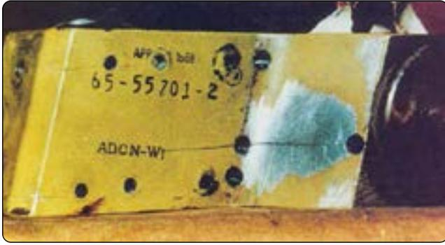
**Figure 8-16.** *Stress corrosion cracking.*
