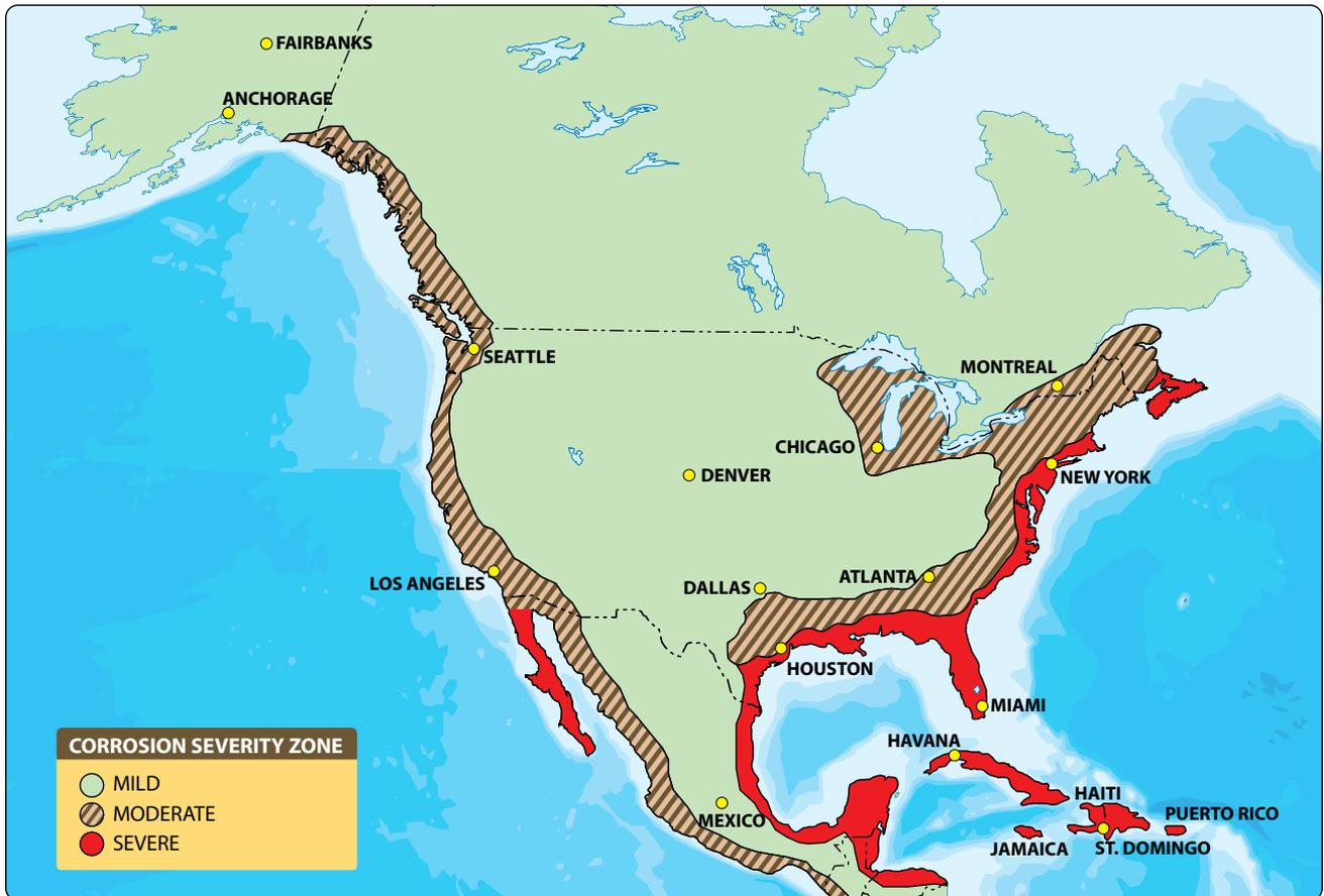
Figure 8-3. North America corrosion severity chart.
