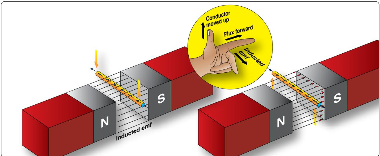
Figure 12-106. An application of the generator left-hand rule.
