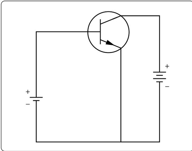
Figure 12-222. NPN transistor.
