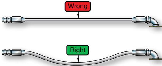
1. Provide slack or bend in the hose line to provide for changes in length that will occur when pressure is applied.
