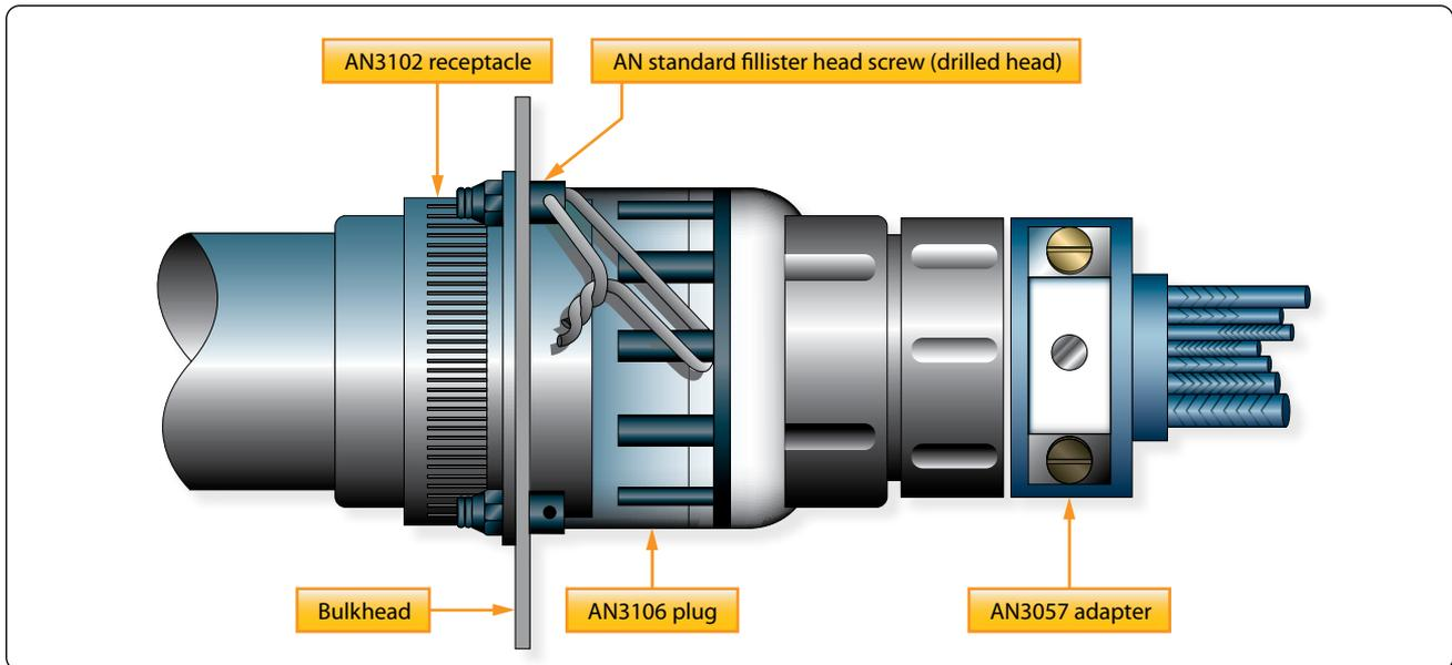
**Figure 7-74.** Safety wiring attachment for plug connectors.
