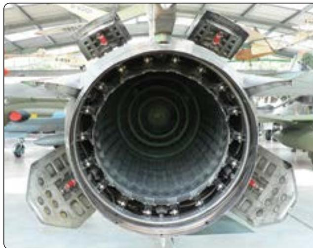
**Figure 8-19.** Exhaust nozzle area.
