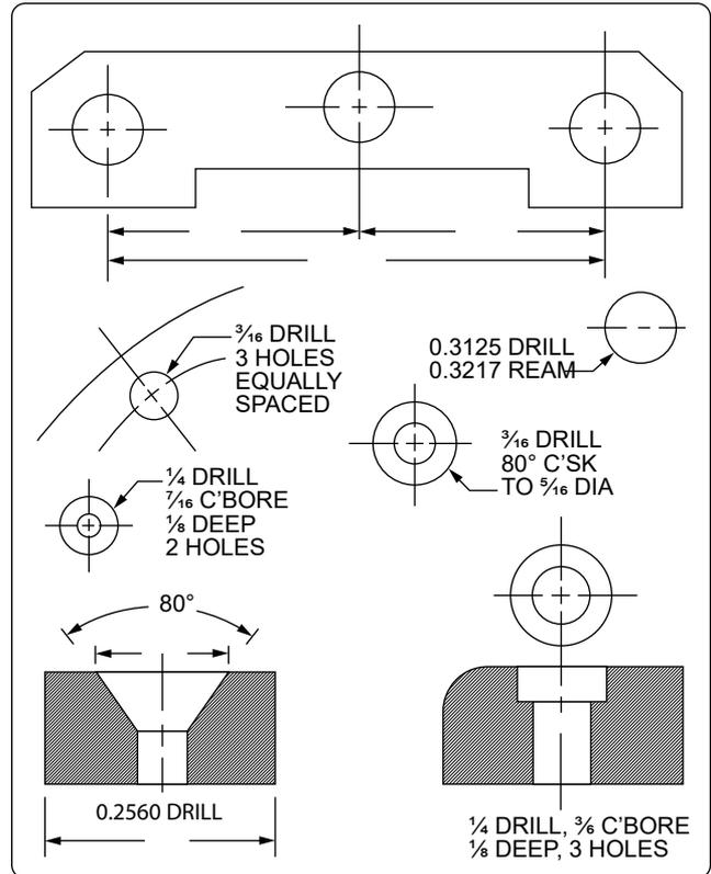
**Figure 4-26.** *Dimensioning holes.*
