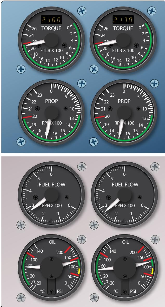
Figure 1-15. Typical examples of turboprop instruments.
