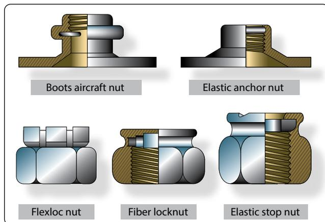
Figure 7-26. Self-locking nuts.
