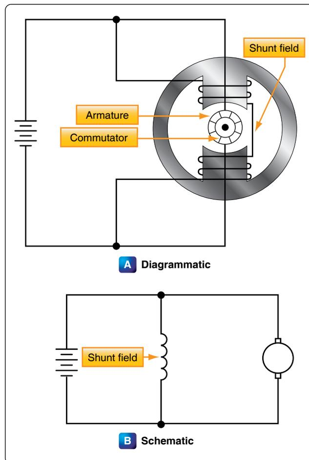
Figure 12-300. Shunt motor.
