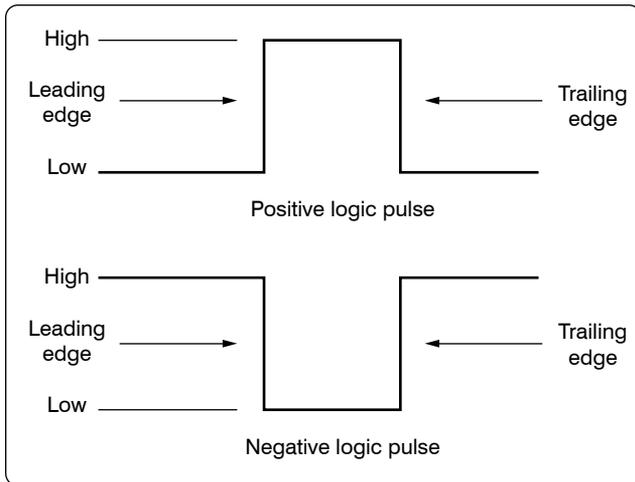
**Figure 12-251.** Positive and negative pulse in an idealized form.
