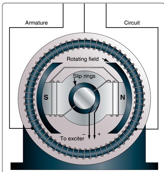
Figure 12-318. Alternator with stationary armature and rotating field.
