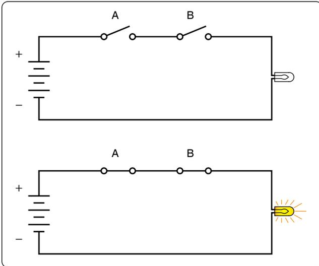
**Figure 12-256.** Simplified diagram of the AND logic.
