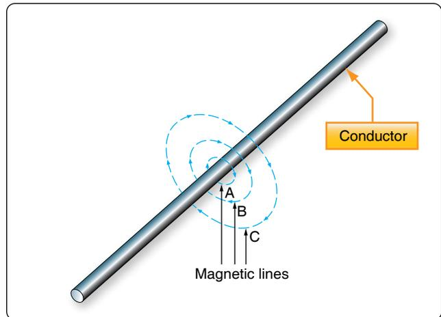
Figure 12-27. Expansion of magnetic field as current increases.
