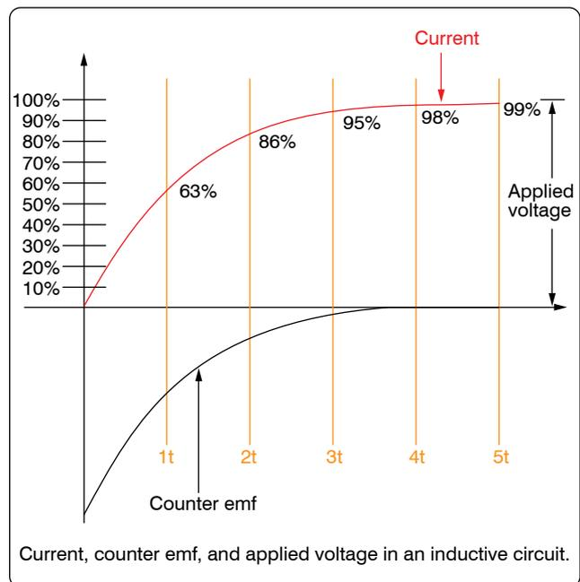
Figure 12-126. Inductor curve.
