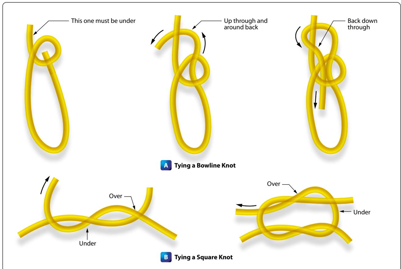
Figure 1-10. Knots commonly used for aircraft tie-down.
