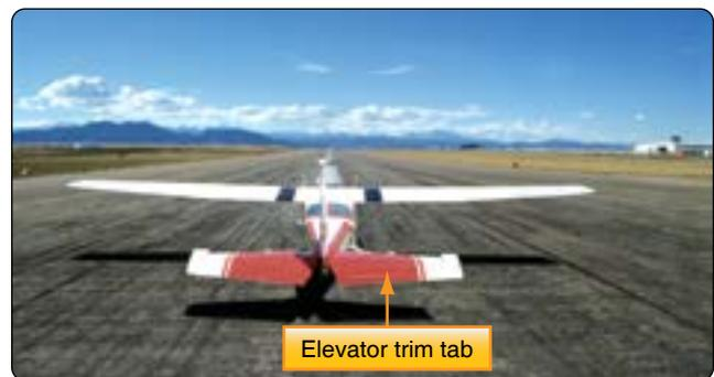
**Figure 5-71.** Elevator trim tab on a Cessna 182.
