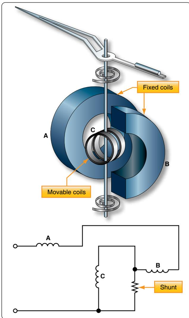
Figure 12-160. Simplified diagram of an electrodynamicometer movement.
