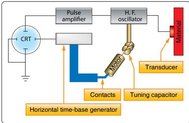
**Figure 10-24.** Block diagram of resonance thickness measuring system.
