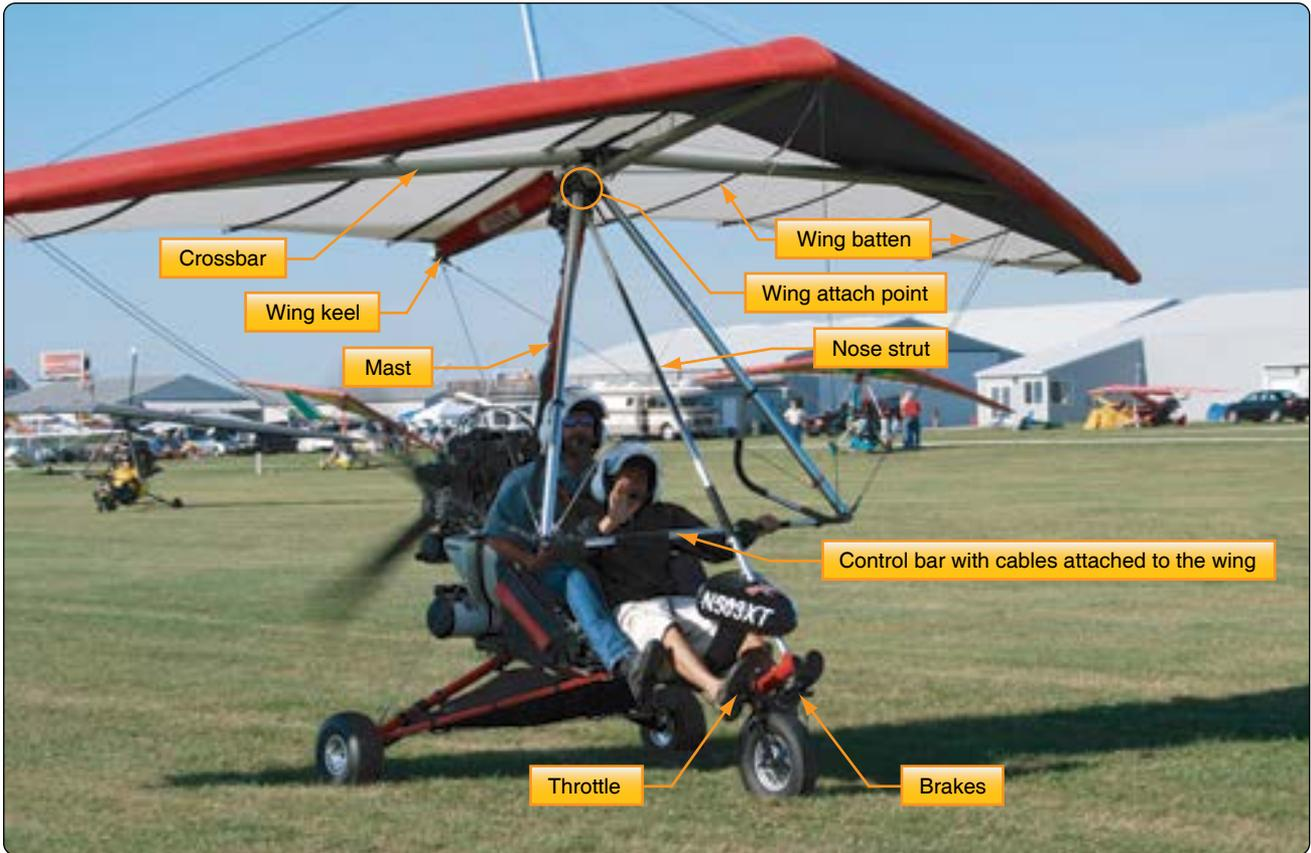
**Figure 5-98.** Weight-shift control aircraft getting ready for flight.
