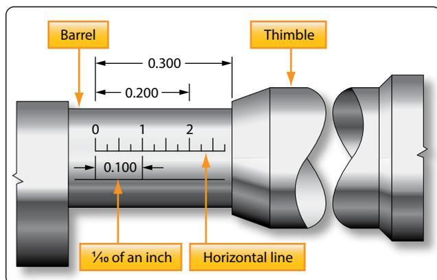
Figure 11-37. Micrometer measurements.
