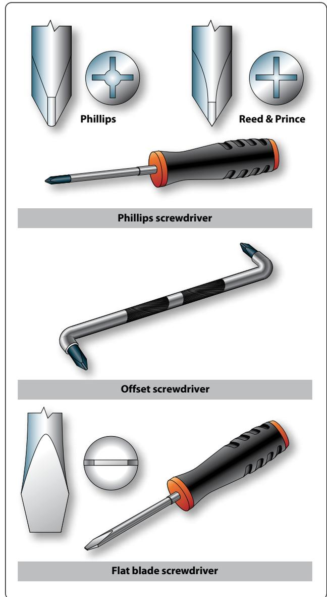
Figure 11-2. Typical screwdrivers.
