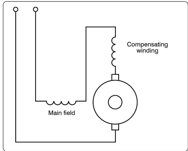
Figure 12-314. Conductively compensated armature of AC series motor.
