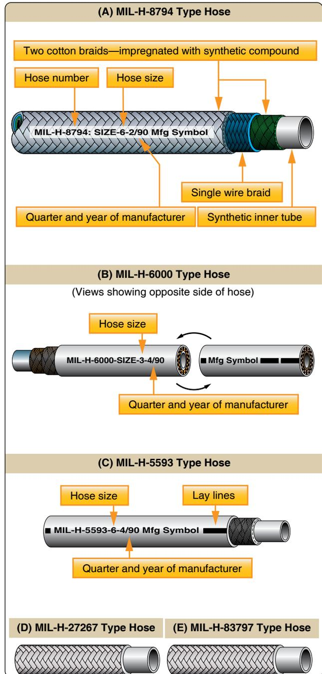
Figure 9-33. Hose identification markings.
