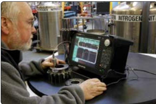
Figure 10-17. Ultrasonic inspection.
