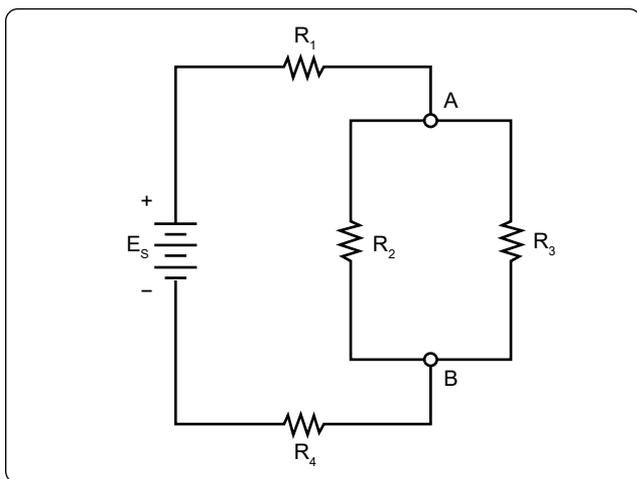
Figure 12-100. Series-parallel circuits.
