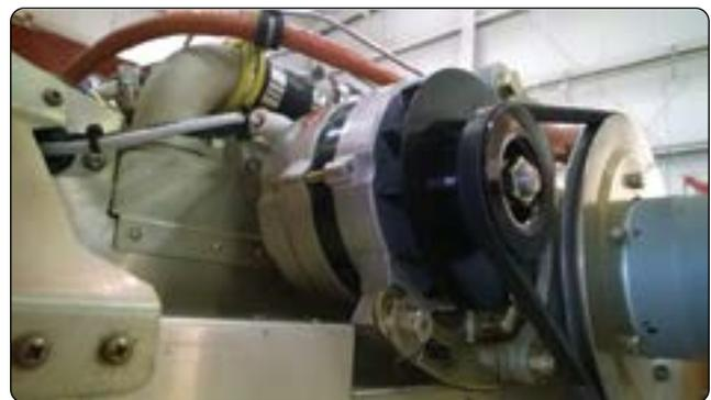
**Figure 12-317.** Belt driven alternator for small single-engine aircraft.
