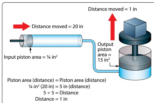
**Figure 5-45.** Piston movement in a hydraulic system.
