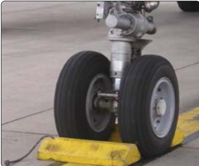
**Figure 1-12.** *Wheels chocked fore and aft.*
