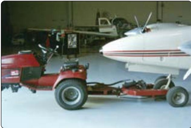
**Figure 1-21.** Typical smaller aircraft tow tractor.
