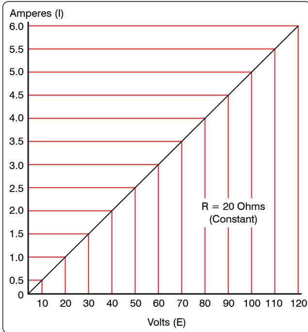
Figure 12-39. Voltage vs. current in a constant-resistance circuit.
