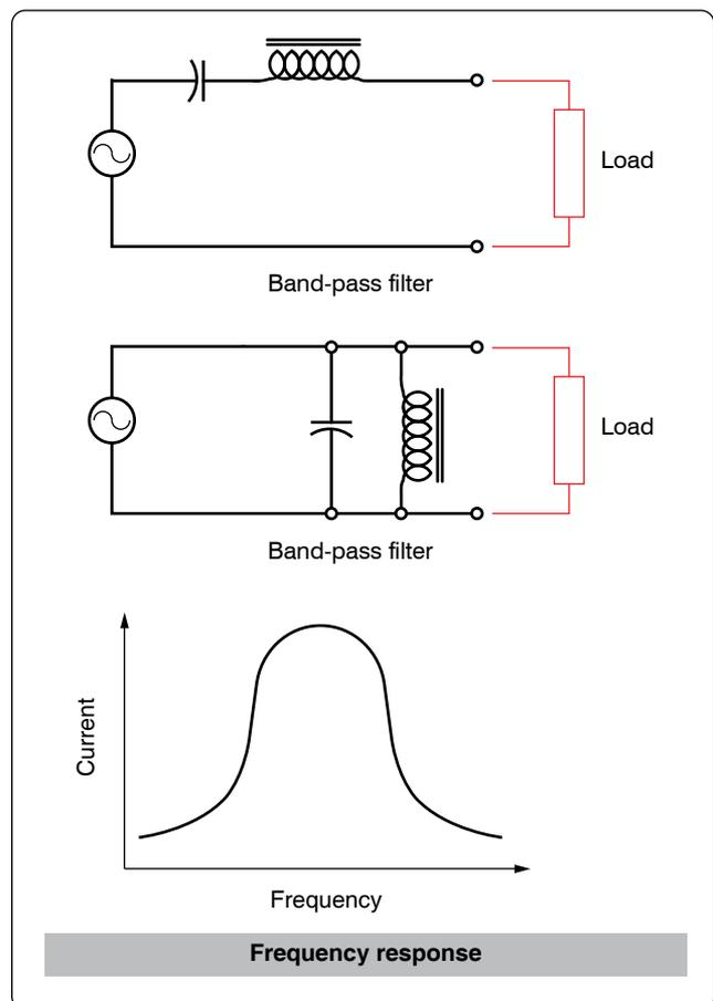
Figure 12-236. Band-pass filter.
