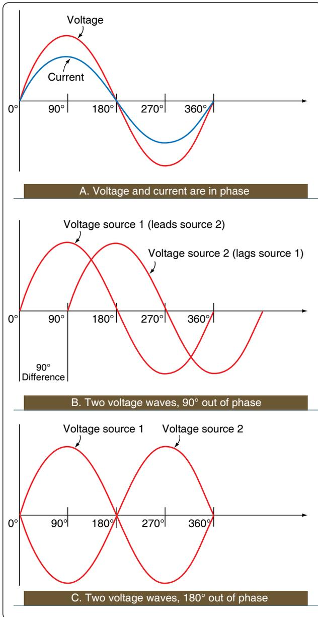
**Figure 12-112.** *In phase and out of phase conditions.*
