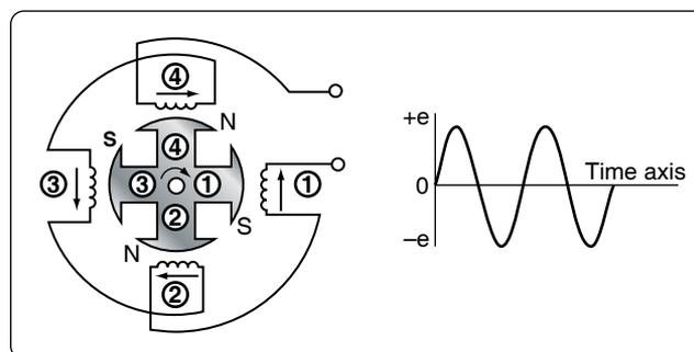
Figure 12-319. Single-phase alternator.
