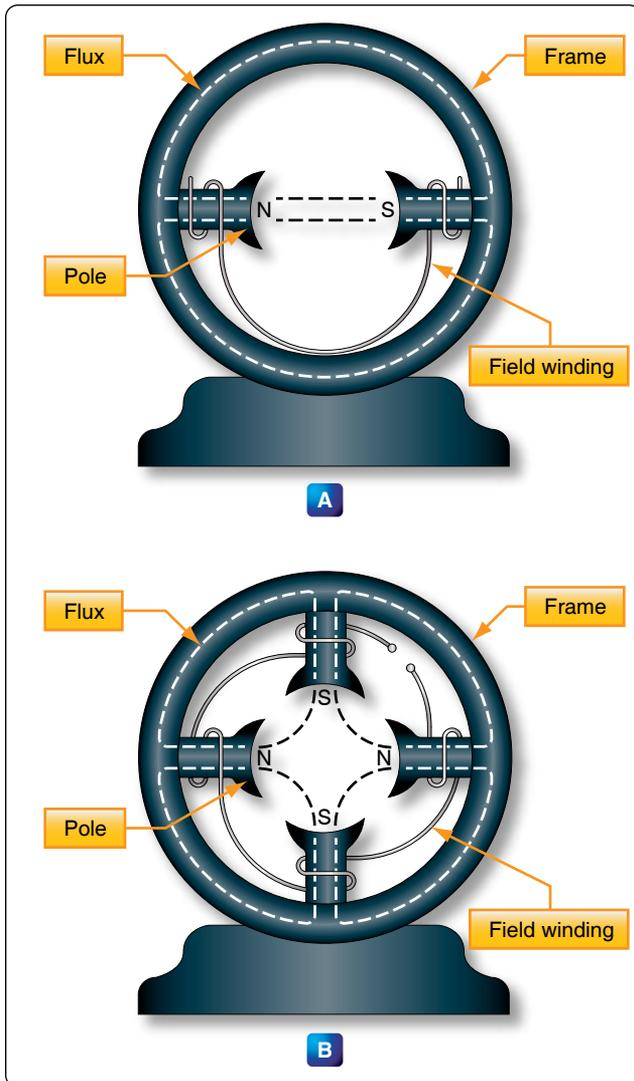
Figure 12-278. A two-pole and a four-pole frame assembly.
