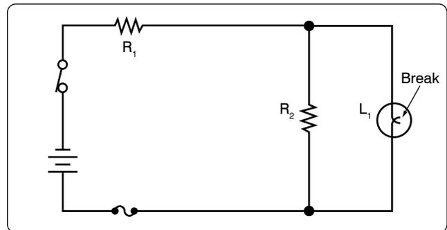
**Figure 12-189.** An open lamp in a series-parallel circuit.
