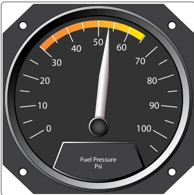
Figure 5-34. Psig read on a fuel pressure gauge.
