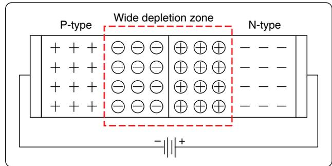
**Figure 12-213.** Reversed diode.
