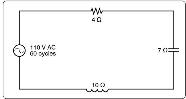
**Figure 12-137.** A circuit containing resistance, inductance, and capacitance.
