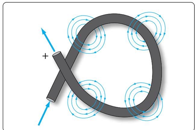
**Figure 12-31.** *Magnetic field around a looped conductor.*
