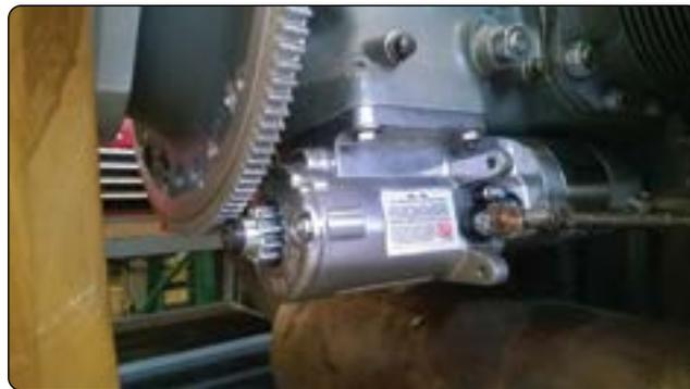
Figure 12-290. DC series starter motor.
