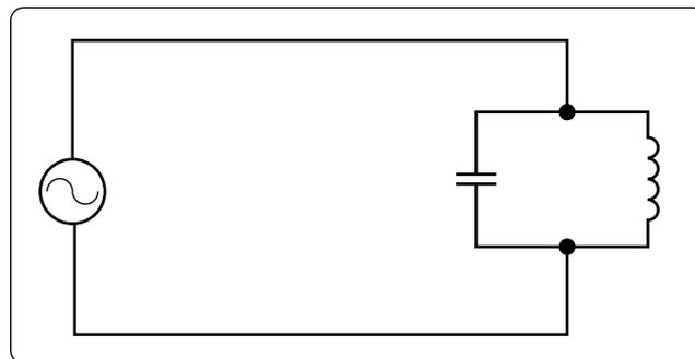
**Figure 12-140.** A parallel resonant circuit.
