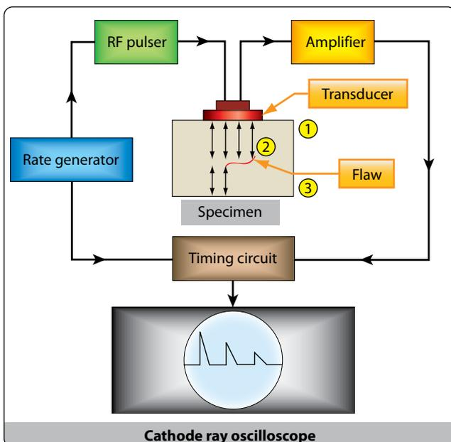
Figure 10-20. Block diagram of basic pulse-echo system.
