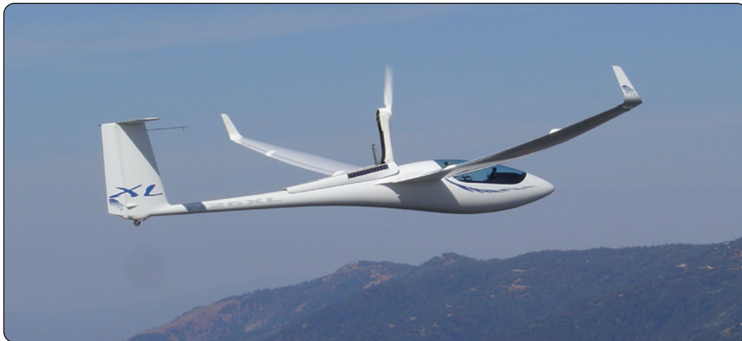
Figure 1-4. An ASH 26 E self-launching motor glider with the propeller extended.
