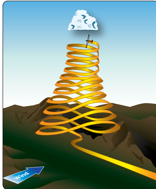
Figure 10-22. One technique for catching a thermal from ridge lift.
