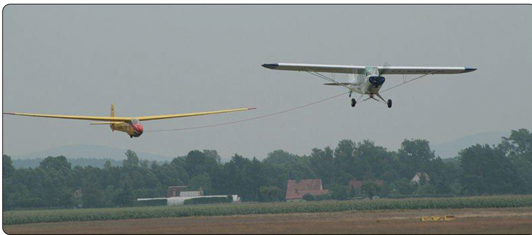
Figure 12-1. Gliders commonly use tow planes to launch and obtain altitude.
