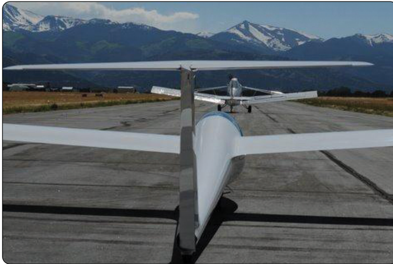
Figure 12-5. The tow pilot advances the throttle smoothly and quickly in one motion so that the glider does not overrun the tow line.
