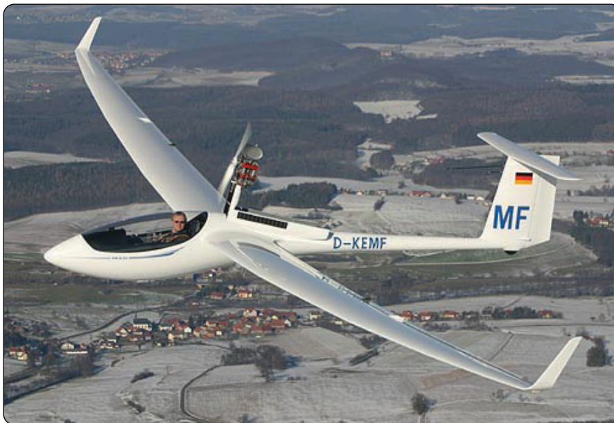
Figure 2-11. A Schleicher ASG-29 E with gasoline sustainer engine mast extended.
