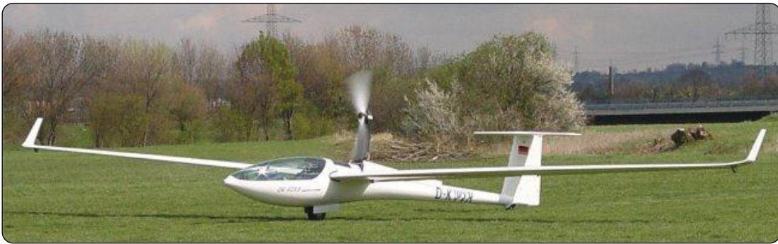
Figure 2-10. A DG-808B 18-meter high-performance glider in self-launch.
