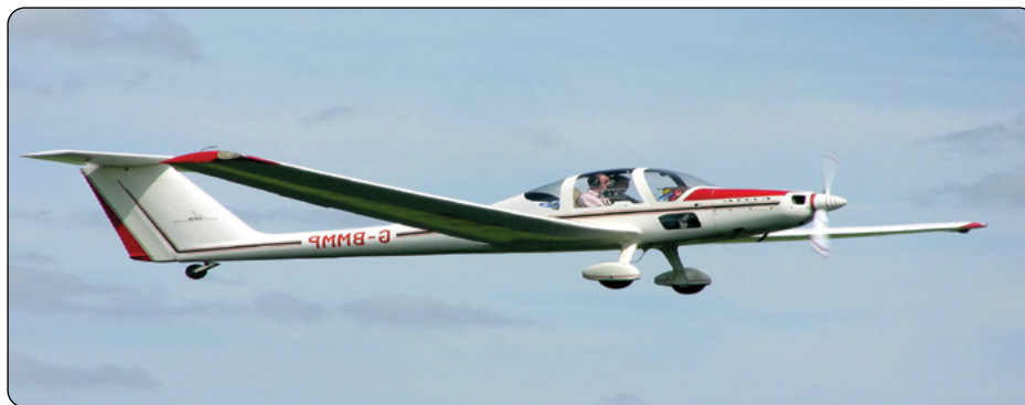
Figure 2-9. A Grob G109B touring motor glider.
