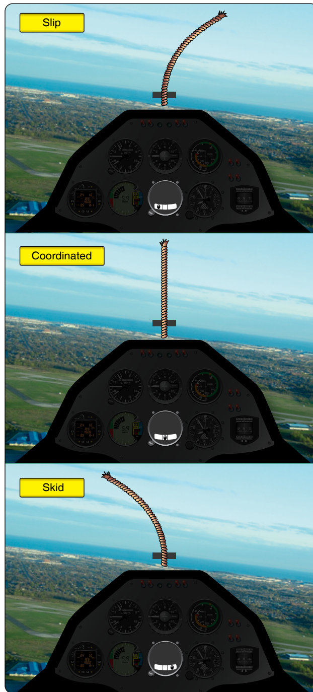
Figure 4-28. Left turn condition indications of a yaw string and inclinometer.
