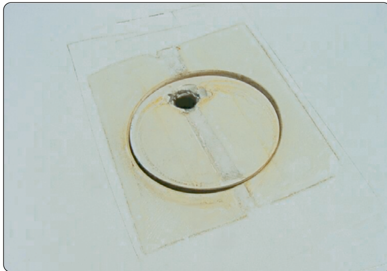
Figure 5-20. Water ballast tank vented filler cap.
