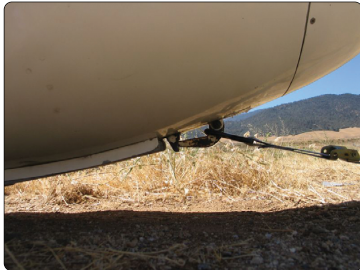
Figure 6-13. Schweizer-type tow hook.
