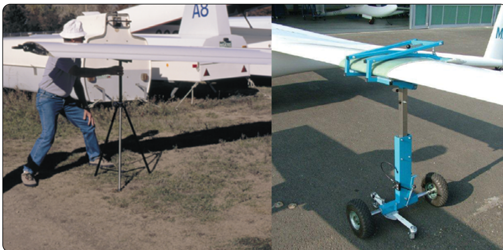
Figure 6-1. Wing stands and wing dollies may assist assembling the glider.
