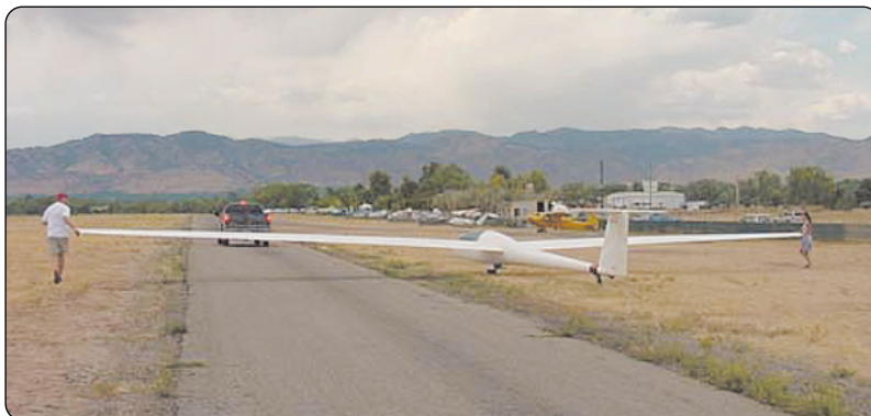
Figure 6-6. Positioning the glider for the tow vehicle.
