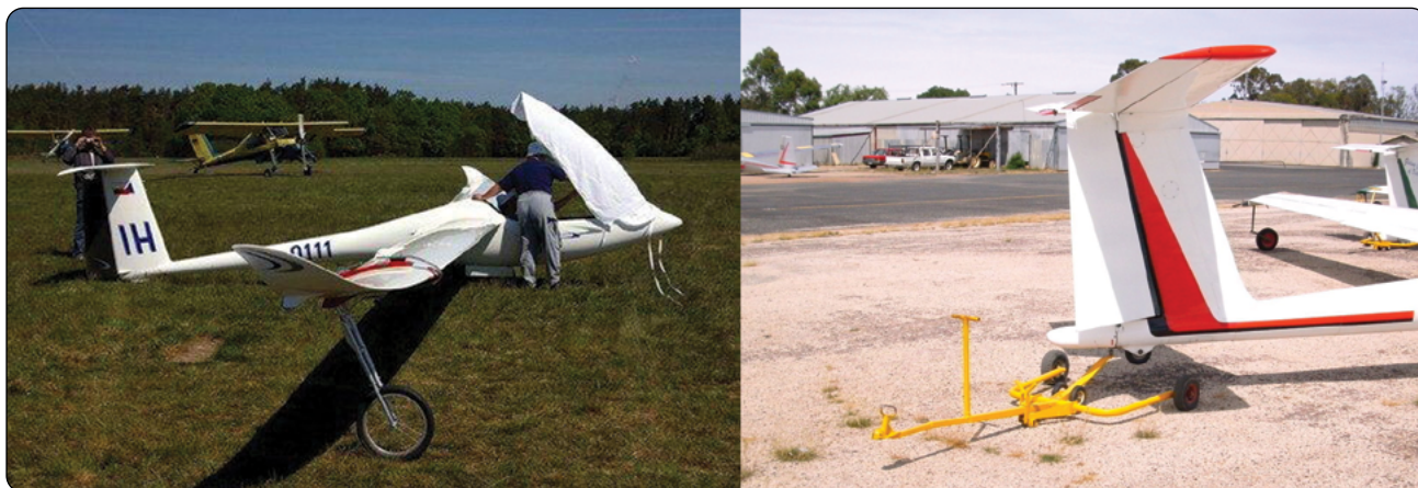
Figure 6-7. A wing dolly (left) ready for attachment and a tail dolly (right) being used for glider ground movement.
