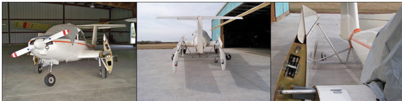
Figure 6-2. Folding the wings of the glider reduces storage space.
