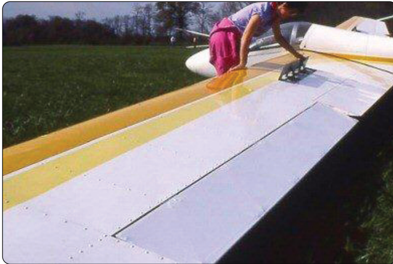
Figure 6-16. Positive control check of spoilers.
