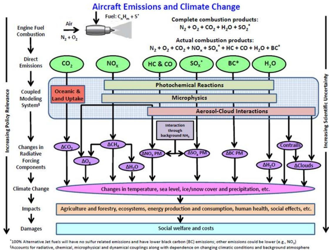
**Figure 7: Schematic representation of emissions from aircraft combustion<sup>53</sup>**
