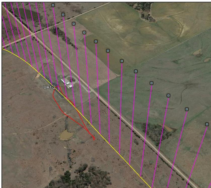
*Figure 11.* Aircraft/UAS telemetry overview presented in Google Earth. Aircraft ground track presented in yellow, with altitude indicated by raised plots; sUAS flight track depicted in red. The participant did not detect the sUAS during this pass. Data derived from Participant 1, Intercept 2. This telemetry corresponds to video data presented in Figure 9.
