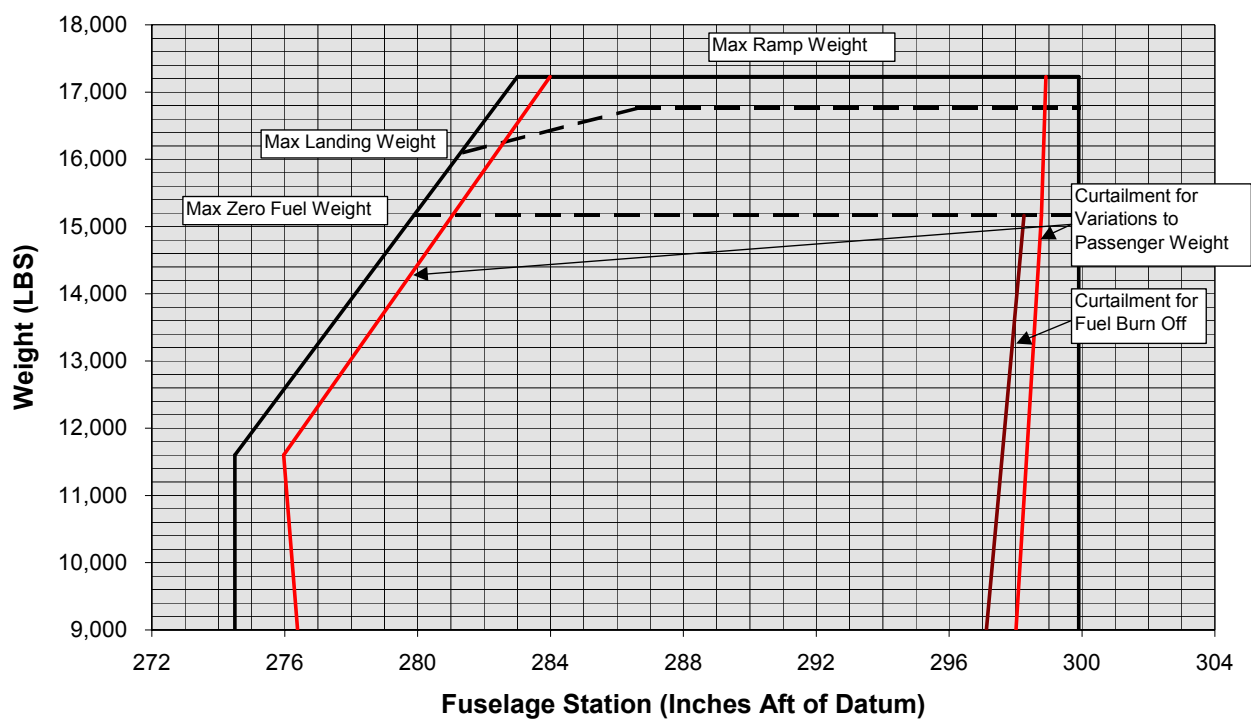
FIGURE 3-3. OPERATIONAL LOADING ENVELOPE USING ACTUAL SEATING LOCATION OF PASSENGERS
