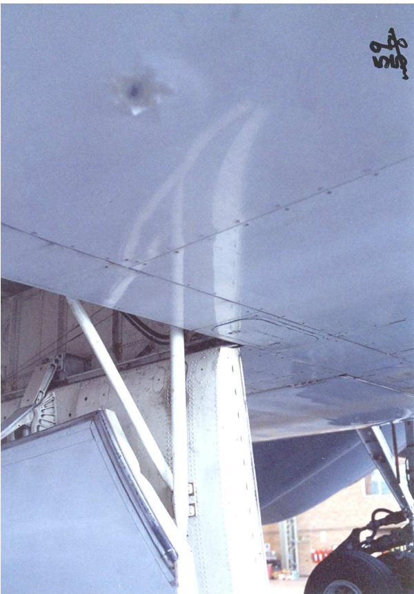
Figure A3.3.7 3" hole in slat (casing uncontained)
