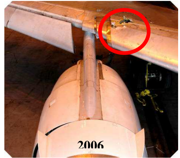
Figure 4.13 Examples of events where disk burst resulted in systems damage which reduced airplane controllability
