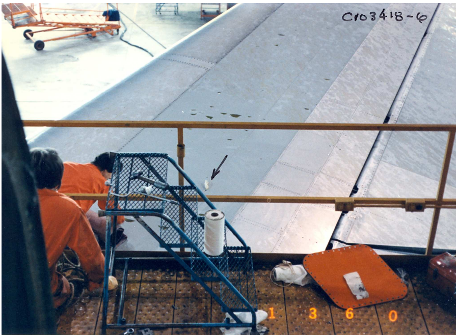
Figure A3.2.10 2" puncture in stabilizer skin (forward arc)
