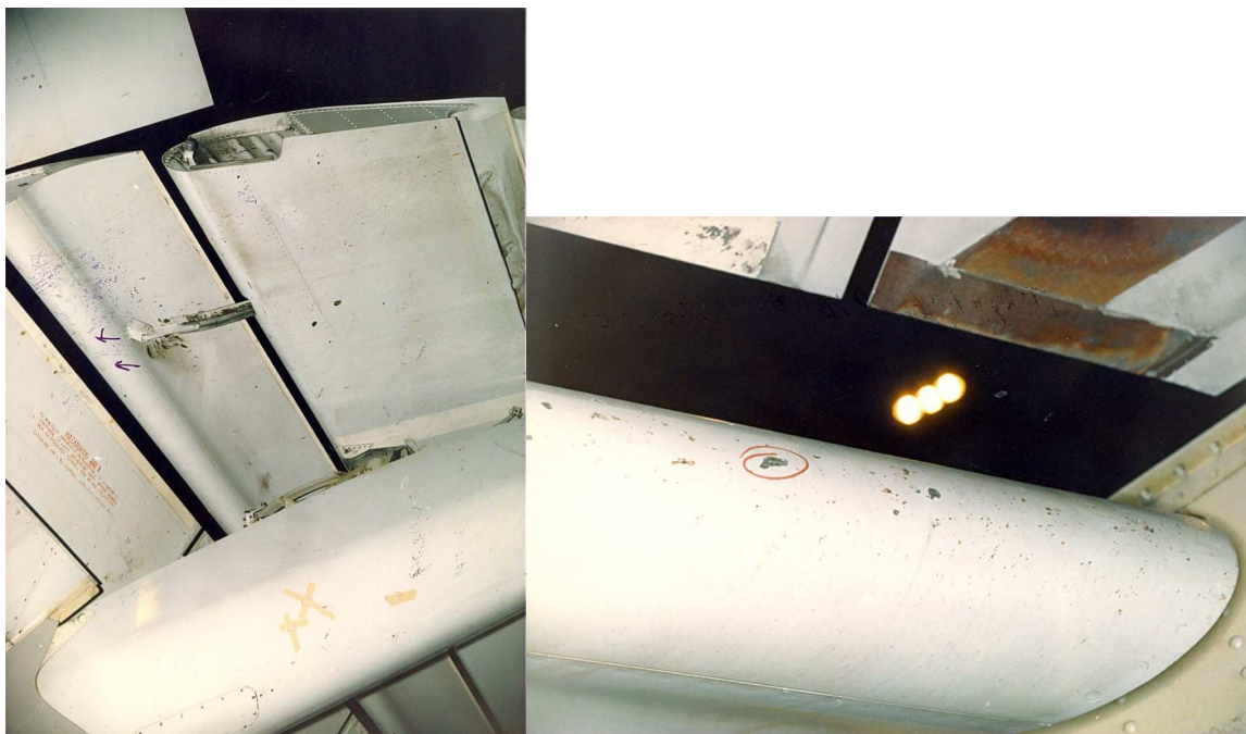
Figure A3.5.4 Nicks and dents to flaps, canoe fairings (tailpipe debris)
