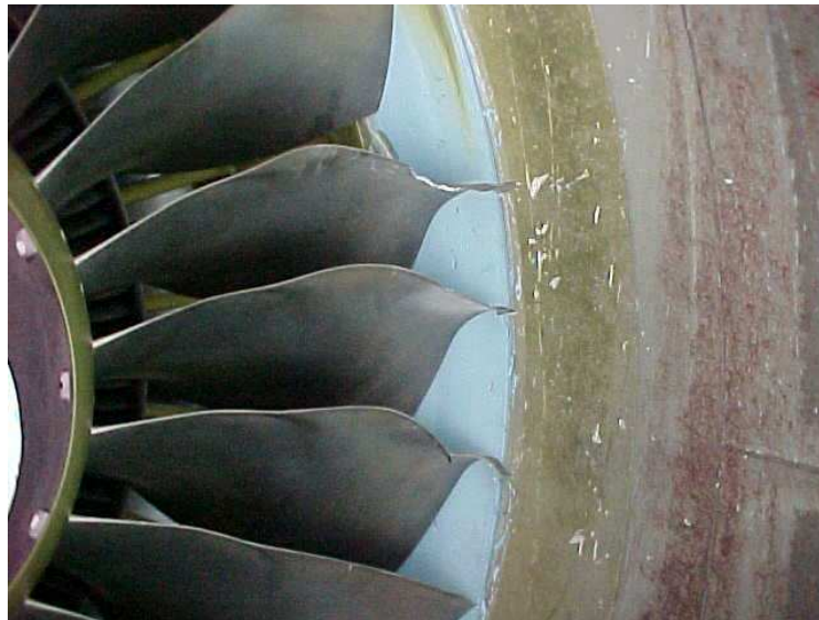
Figure A3.2.5 Wide-chord blade; 8 lb pelican ingestion
