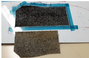
After severe in-flight hail, in about 90 flights significant debonding of metal sandwich face sheets. As a result of cyclic loading on the upper skin panel (internal pressure and aerodynamic suction loading) the crushed core has cracked and eventually it failed leading to the bulged skin observed during flight.
