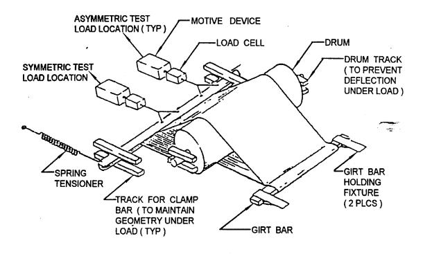
Figure 6 - Typical Girt Loading Test Set-Up
